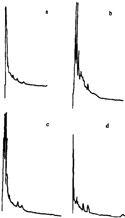
Fig. 2 Selected chromatograms of several samples extracts from the Great Wall bay a. BHCs, DDTs in water; b. BHCs, DDTs in sediment; c. PCBs in sediment; d. PCBs in patella
