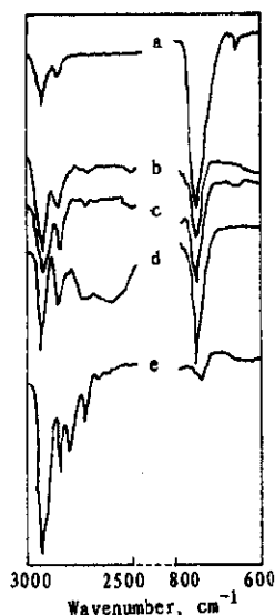
Fig. 5 Different infrared spectra of (a) K^+ , (b) Ca^{2+} , (c) Na^+ , and (d) Cu^{2+} clays treated with piperidine. The spectrum of (e) piperidine as a thin film is also shown
