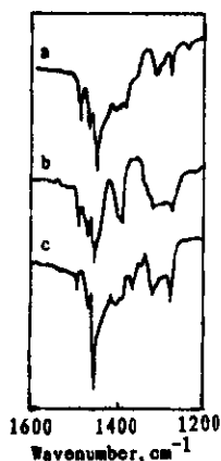
Fig. 3 Different infrared spectra of (a) \text{Fe}^{3+} , and (b) \text{Al}^{3+} homoionic clays treated with dimepiperate, also (c) \text{Al}^{3+} clay treated with piperidine
