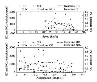
Fig. 3 Pollutant concentrations versus vehicle speed (a) and versus vehicle acceleration (b).
