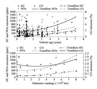
Fig. 2 Pollutant concentrations versus vehicle age (a) and versus odometer reading (b).
