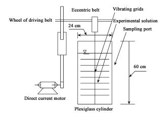
Fig. 1 Turbulence simulation tank (TST).
