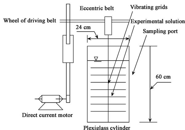
Fig. 1 Turbulence simulation tank (TST).
