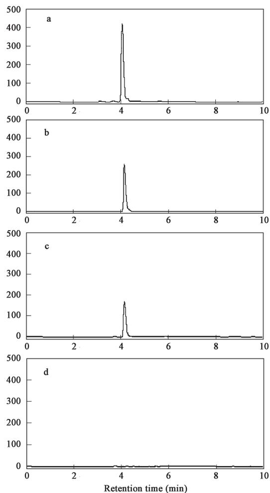
Fig. 3 HPLC profiles for the biodegradation of MP by the enzymes of *A. radioresistens* USTB-04 in different reaction periods. (a) 0 h; (b) 0.3 h; (c) 2.0 h; (d) 15.0 h.
