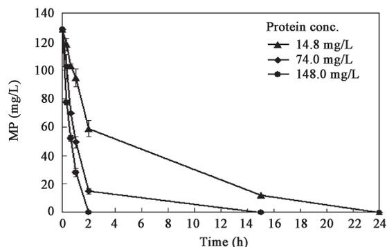
Fig. 2 Biodegradation of MP by the enzymes of *A. radioresistens* USTB-04 with different protein concentrations at 30°C and pH 7.0.
