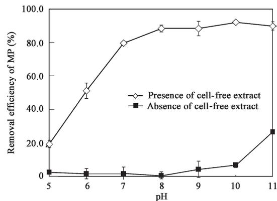
Fig. 4 Effects of pH on the biodegradation of MP by the enzymes of *A. radioresistens* USTB-04.
