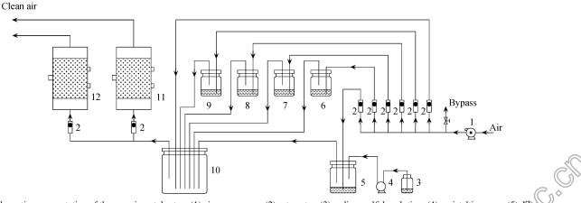
**Fig. 1** Schematic representation of the experimental setup. (1) air compressor; (2) rotameter; (3) sodium sulfide solution; (4) peristaltic pump; (5) diluce  $H_2SO_4$  solution; (6) pure ammonial solution; (7) pure ethyl mercaptan solution; (8) pure butyric acid solution; (9) pure styrene solution; (10) mixing chamber; (11) neutral pH biofilter; (12) low pH biofilter.
