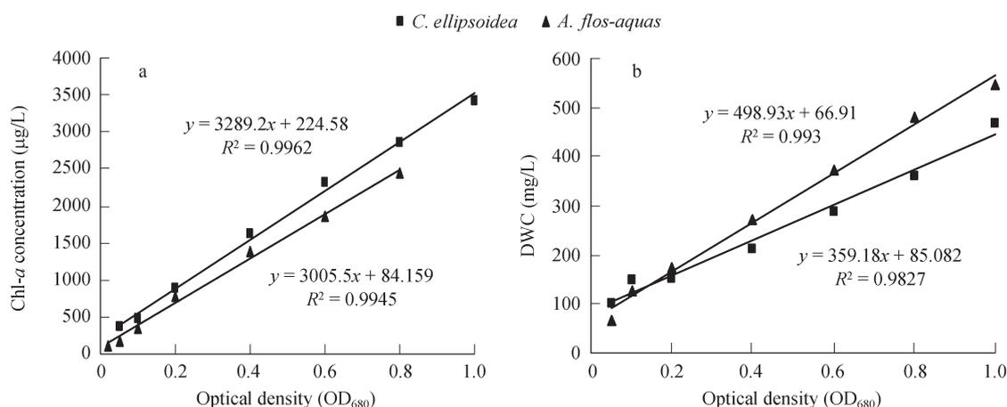
Fig. 1 Relationship between  $\text{OD}_{680}$  and chl-*a* (a), dry weight (b).
