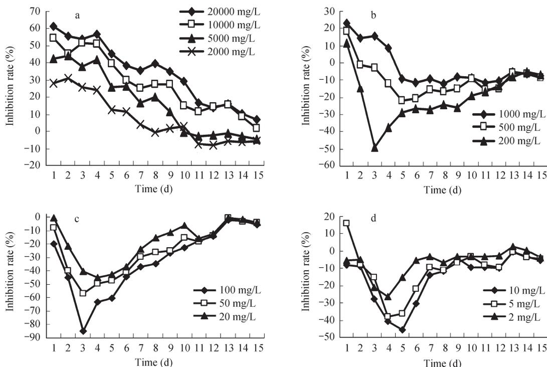
Fig. 3 Inhibition of *A. flos-aquae* by different MTBE concentrations.
