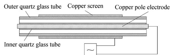
Fig. 2 Schematic of non-thermal plasma (NTP) reactor. Inner tube: 5 mm inner diameter and 8 mm outer diameter; outer tube: 22 mm inner diameter and 25 mm outer diameter.
