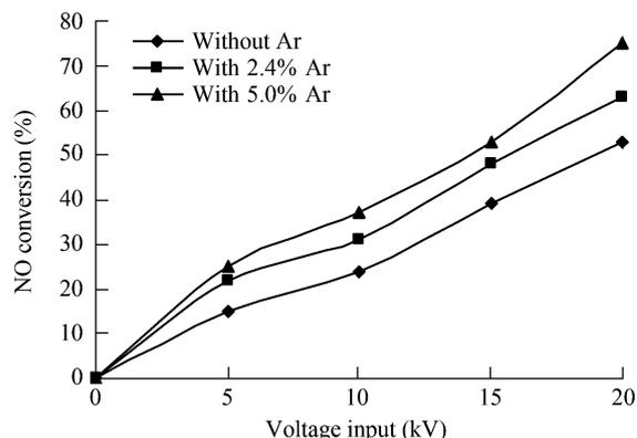
Fig. 3 Effect argon additive on the conversion of NO in  $N_2/O_2/argon$  plasma system.
