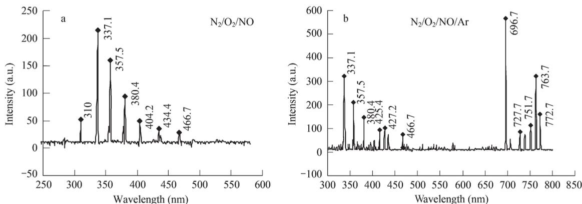
Fig. 4 Effect of argon additive on the emissive spectra for N<sub>2</sub>/O<sub>2</sub>/NO plasma system (a) and N<sub>2</sub>/O<sub>2</sub>/NO/argon plasma system (b).
