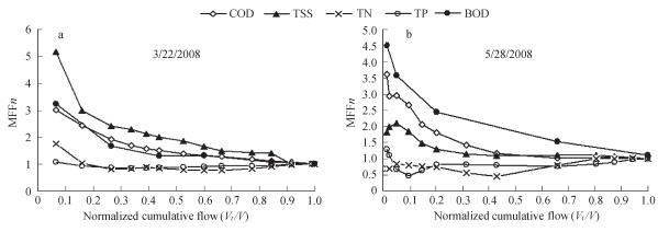
**Fig. 5** Values of  $MFF_n$  in two typical rainfall events.
