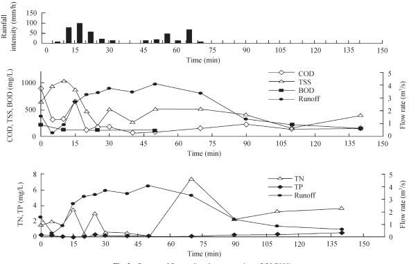
Fig. 2 Process of flow and total concentrations (5/28/2008).
