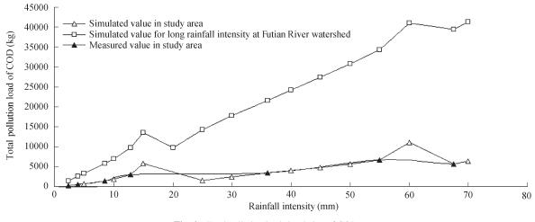
Fig. 4 Total pollution load simulation of COD.
