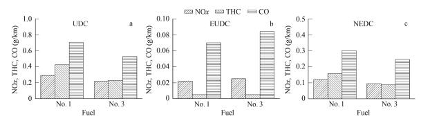
Fig. 4 Effect of hydrocarbon compositions on tailpipe emissions over UDC (a), EUDC (b), and new European driving cycle (NEDC) (c) cycles.
