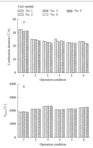
**Fig. 3** Effect of hydrocarbon compositions on combustion duration (a) and  $T_{MAX}$  (b).
