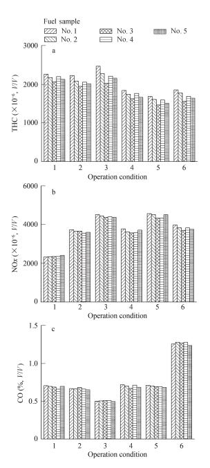
**Fig. 2** Effect of hydrocarbon compositions on engine-out THC (a), NO*x* (b) and CO (c) emissions.
