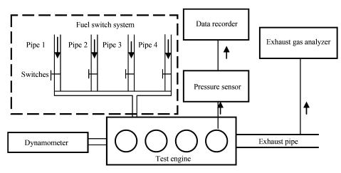
Fig. 1 Schematic of the engine test bench.
