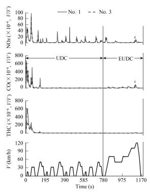
Fig. 5 Real time tailpipe emissions over NEDC cycle.
