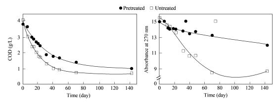
Fig. 5 Influence of wastewater pre-treatment by air on the COD-conversion (a) and the decrease of absorbance at 270 nm (b) during the subsequent methanogenic fermentation.
