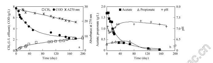
Fig. 1 Kinetics of COD-removal, absorbance at 270 nm (A270 nm), cumulative formation of methane (a) and the degradation kinetics of fatty acids related to the changes of pH (b).
