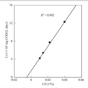
Fig. 2 Lineweaver-burk-plot of maximal COD-conversion rates against the wastewater concentration.
