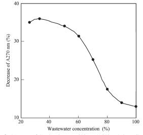
**Fig. 3** Decrease of the absorbance at 270 nm (A270 nm) depending on the wastewater concentration after the methanogenic fermentation.
