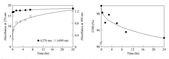
Fig. 4 Changes of the absorbance at 270 and 490 nm (a) and COD (b) of the wastewater depending on the duration of air exposition.
