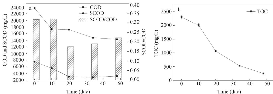
Fig. 2 Variations of COD, SCOD, SCOD/COD and TOC during anaerobic digestion.
