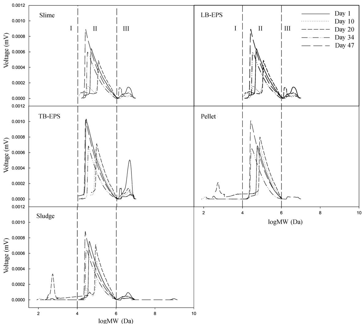
**Fig. 4** Gel permeation chromatograms (GPC) of dissolved organic matters (DOM) in extracellular polymeric substances (EPS) matrix and the sonicated sludge flocs during anaerobic digestion.
