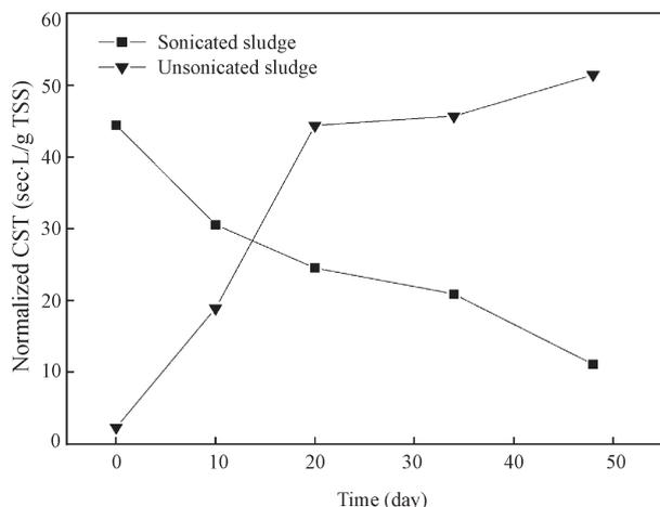
Fig. 6 Variations of the normalized CST during anaerobic digestion.
