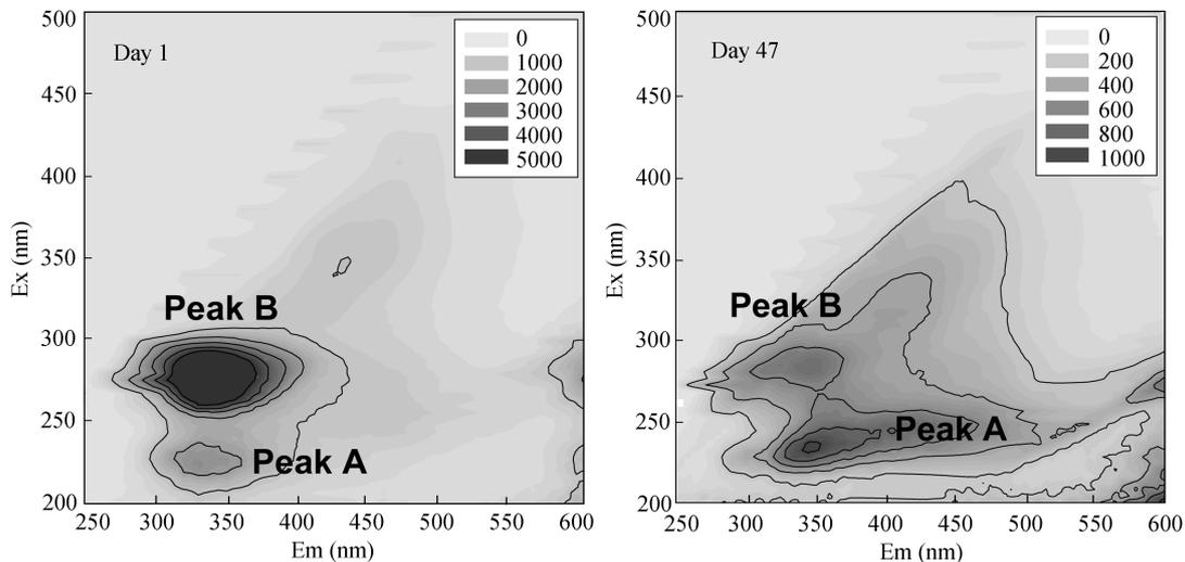
**Fig. 5** Typical excitation-emission matrix (EEM) spectroscopy of loosely bound EPS (LB-EPS) fraction for the sonicated sludge.
