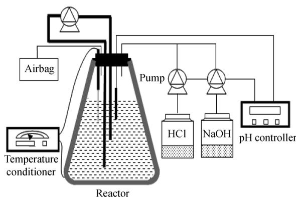
Fig. 1 Schematic diagram of anaerobic digestion.
