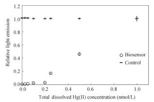
**Fig. 1** Typical [Hg(II)] response by biosensor and constitutive control in M9NO<sub>3</sub> medium. *Y*-axis is ratio of  $I_B$  or  $I_C$  at each Hg standard concentration and at [Hg(II)] = 1.0 nmol/L (max  $I_B$  = 654 RLU;  $I_C$  = 1.4 RLU). Error bars are SE of ANOVA-derived means.
