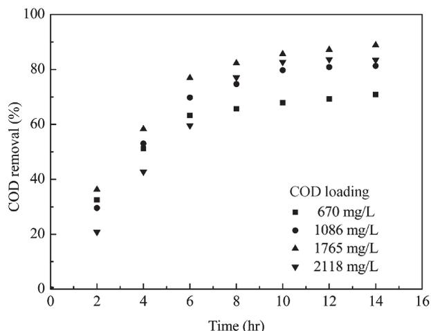
**Fig. 5** COD removal during the aeration time under different COD loadings at pressure 0.30 MPa, aeration rate  $25 \text{ m}^3/(\text{m}^3 \cdot \text{hr})$ , MLSS 6 g/L.
