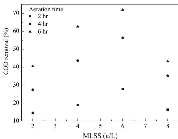
**Fig. 6** COD removal change with MLSS at pressure 0.30 MPa, aeration rate  $25 \text{ m}^3/(\text{m}^3 \cdot \text{hr})$ .
