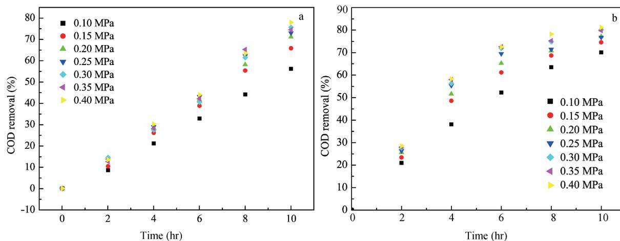
**Fig. 2** COD removal vs. the aeration time at different pressures and MLSS. (a) aeration rate  $25 \text{ m}^3/(\text{m}^3 \cdot \text{hr})$ , MLSS  $2 \text{ g/L}$ ; (b) aeration rate  $25 \text{ m}^3/(\text{m}^3 \cdot \text{hr})$ , MLSS  $6 \text{ g/L}$ .
