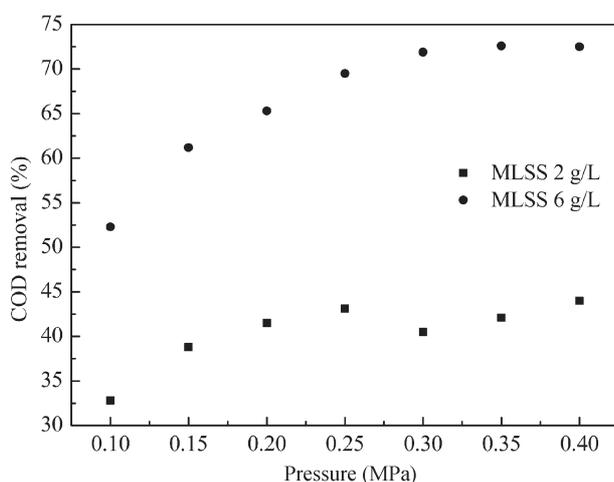
**Fig. 3** COD removal vs. pressures at the aeration time  $6 \text{ hr}$  and aeration rate  $25 \text{ m}^3/(\text{m}^3 \cdot \text{hr})$ .
