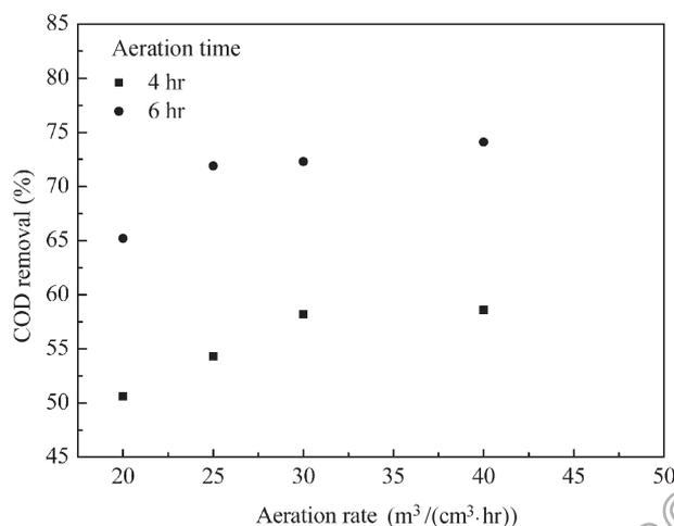
**Fig. 4** COD removal during the aeration process for different aeration rates at pressure  $0.30 \text{ MPa}$ , MLSS  $4 \text{ g/L}$ .
