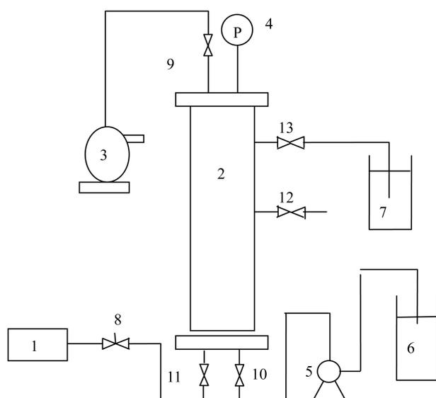
**Fig. 1** Schematic flow diagram of the pressurized activated sludge process. (1) compressor; (2) pressurized bioreactor; (3) flow meter; (4) pressure gauge; (5) pump; (6) influent tank; (7) effluent tank; (8) redactor; (9) outlet air valve; (10) inlet water valve; (11) inlet air valve; (12) sampling valve; (13) effluent valve.
