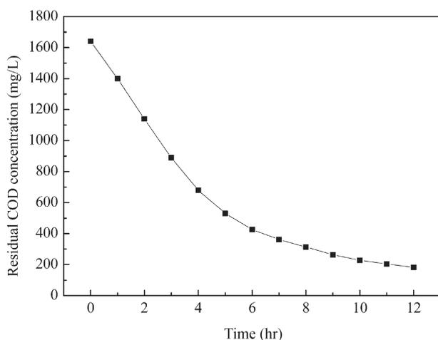
**Fig. 8** Mixed liquor COD removal during the aeration process. Operation condition: influent COD: 2500–5000 mg/L; 0.30 MPa; MLSS: 4.12 g/L; aeration time: 6 hr; aeration rate: 25 m<sup>3</sup>/(m<sup>3</sup>·hr).
