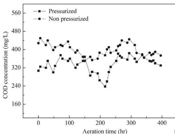
**Fig. 7** Treatment effect comparability between the pressurized activated sludge and non-pressurized activated sludge.
