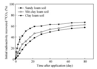
Fig. 2 Mineralization of  $^{14}$ C-glyphosate to  $^{14}$ CO<sub>2</sub> in three soils incubated at 20°C.
