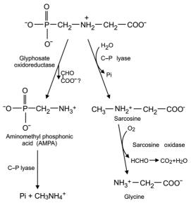
Fig. 5 Microbial degradation of glyphosate in soil through sarcosine or AMPA (Liu et al., 1991).
