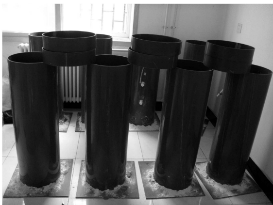
Fig. 1 Design of the experimental facility for quantifying methane emissions from manure storage.
