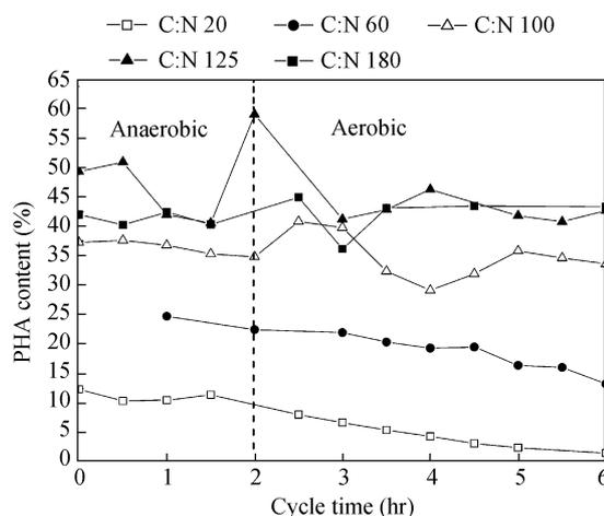
Fig. 5 Profile of PHA production at different C:N weight ratios in one cycle.
