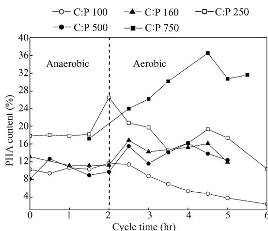
**Fig. 2** Profile of PHA production at different C:P weight ratios in one cycle.
