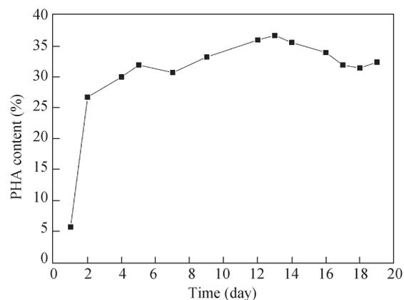
Fig. 4 Profile of PHA production in 2#SBR during the acclimation phase for nitrogen limitation.
