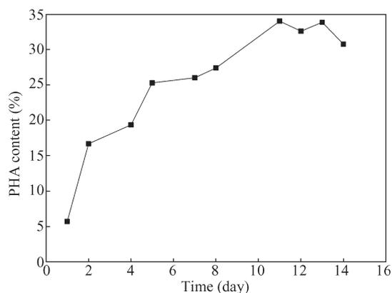
**Fig. 1** Profile of PHA production in 1#SBR during the acclimation phase for phosphorus limitation.
