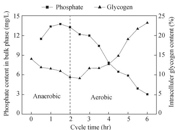
Fig. 3 Contents of glycogen and phosphorus in biomass in 1#SBR at C:P (W/W) 160.
