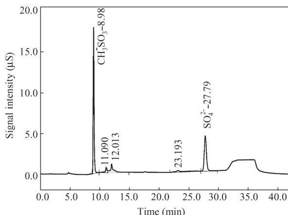
**Fig. 5** Example of chromatogram demonstrating the detection and resolution of IC measurement of  $\text{CH}_3\text{SO}_3^-$  and  $\text{SO}_4^{2-}$  in samples collected the suspended particles.
