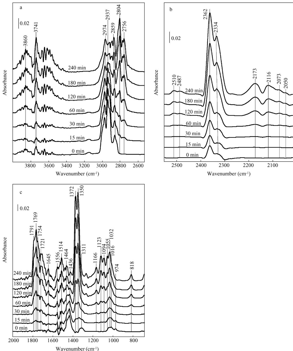
**Fig. 2** *In situ* FT-IR spectra of the UV-induced degradation of odorous DMS in the wavenumbers of 4000–2530  $\text{cm}^{-1}$  (a), 2600–2000  $\text{cm}^{-1}$  (b), and 2000–680  $\text{cm}^{-1}$  (c).
