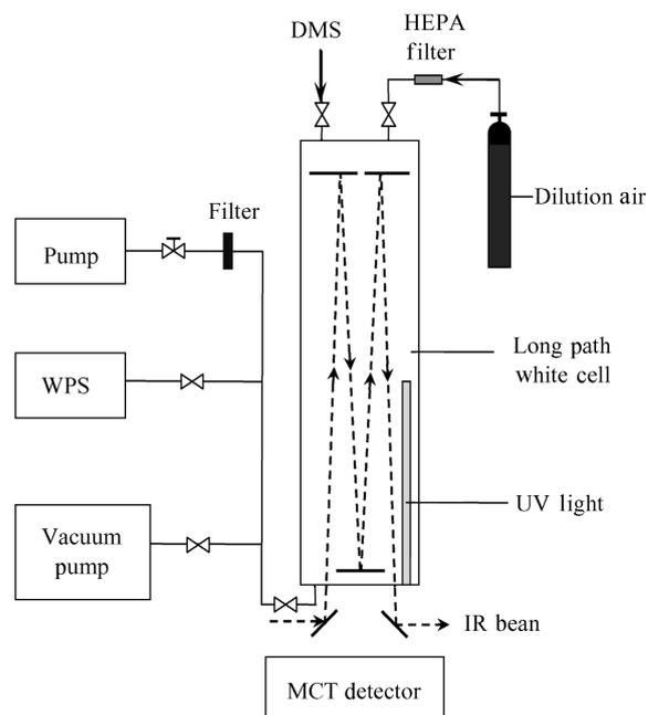
**Fig. 1** Schematic diagram of the apparatus. DMS: dimethyl sulfide; WPS: wide-range particle spectrometer; MCT: mercury-cadmium-telluride.
