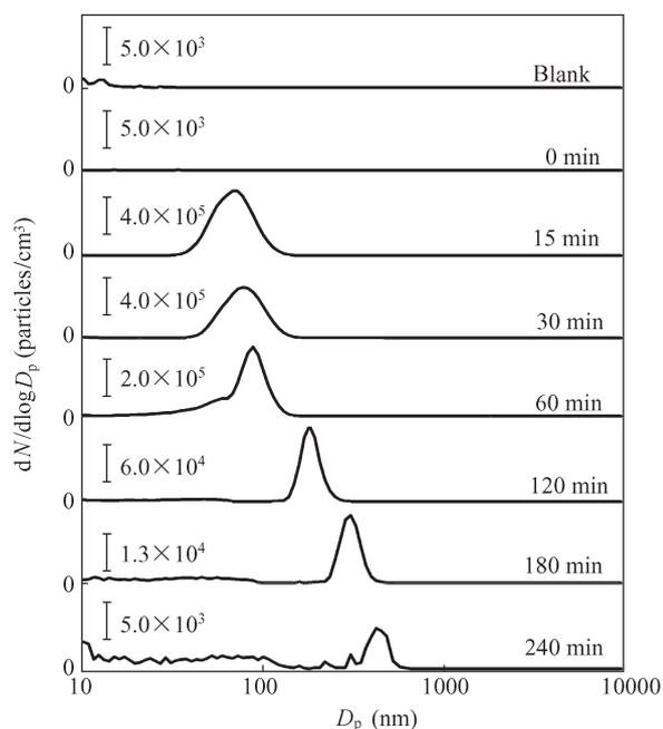
**Fig. 4** Time-series count size distribution of suspended particles ( $D_p$ ) detected accompanying with the degradation of odorous DMS under UV irradiation.
