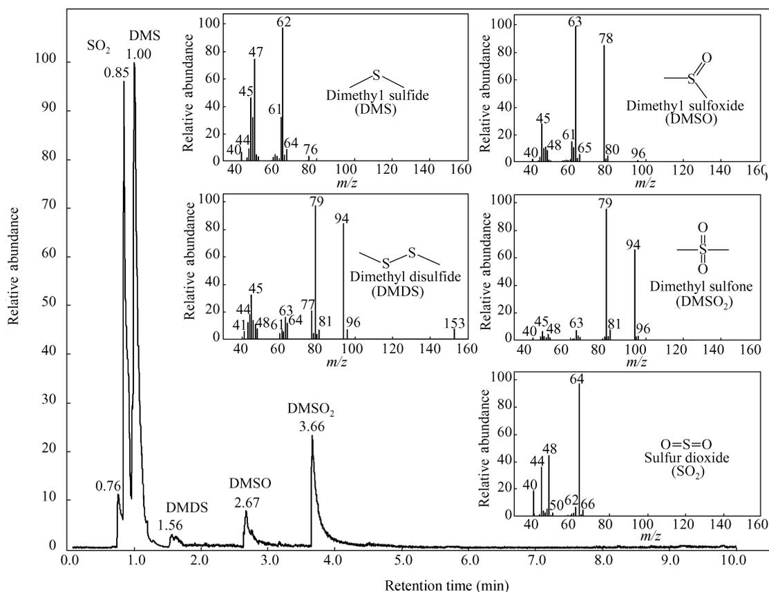
**Fig. 3** GC-MS chromatogram and mass patterns for the intermediates after 240 min of reaction.
