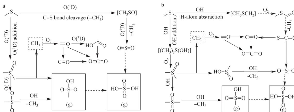
**Fig. 6** Proposed degradation pathways of DMS in the present systems. (a)  $O(^1D)$ -initiated oxidation mechanism; (b) OH-initiated oxidation mechanism.
