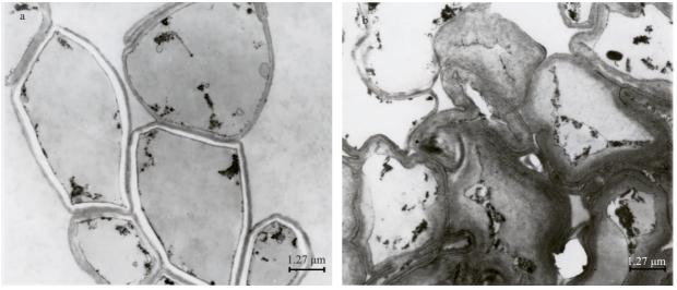
Fig. 4 Transmission electron micrograph of biosorbent P. platypus before (a) and after (b) adsorption of Cd(II).
