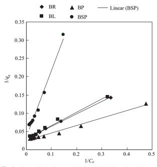
Fig. 2 Langmuir isotherm model for Cd(II) biosorption. BR: raw biosorbent; BL: biosorbent without lipid; BP: biosorbent without lipid and protein; BSP: biosorbent without lipid, protein and soluble polysaccharides. Conditions: pH 6.0, biomass dosage 1 g/L; contact time 6 hr; temperature  $(28 \pm 1)^{\circ}$ C.
