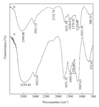
**Fig. 5** FT-IR spectra of biosorbent *P. platypus* before (a) and after (b) Cd(II) adsorption.
