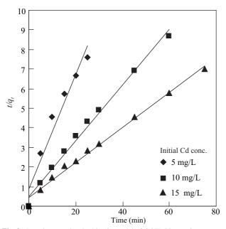
**Fig. 3** Pseudo second-order kinetic model of Cd(II) biosorption onto *P. Platypus.* pH: 6.0; biomass dosage: 1 g/L; contact time: 5–360 min.
