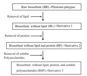
Fig. 1 Scheme for sequential removal of cell wall components of *P. platypus.*
