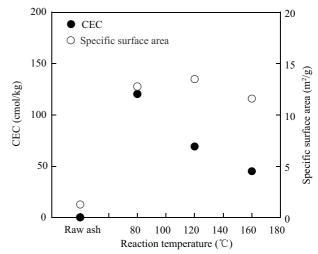
Fig. 2 Specific surface areas and cation exchange capacities (CECs) of PSA and the products obtained at various temperatures of 48-hr reaction.
