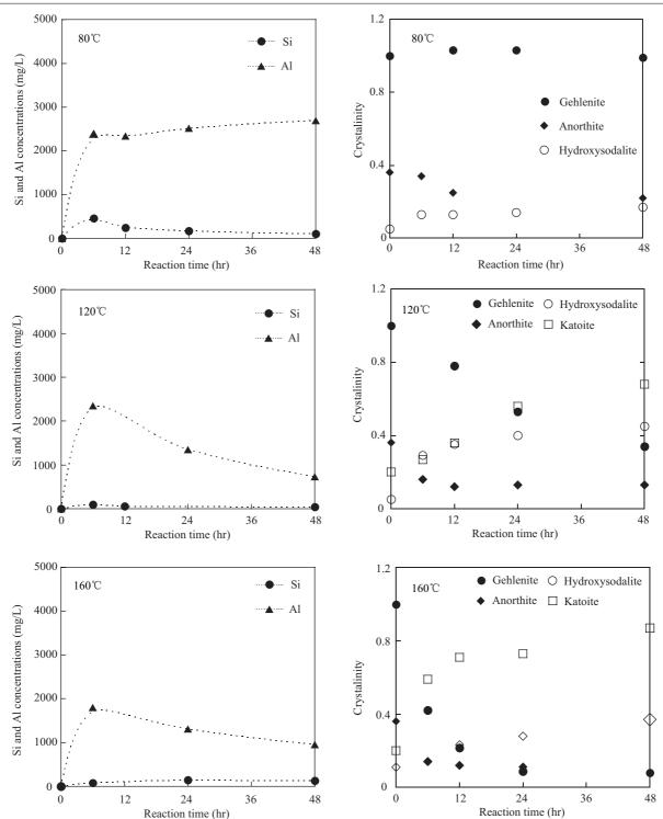
Fig. 4 Si and Al concentrations in the solution and the relative crystallinities of the product phases in the solid during the alkali reaction at 80, 120 and 160°C.
