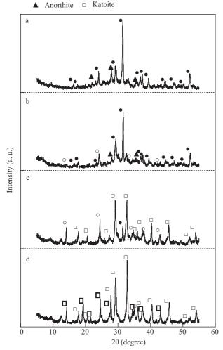
Fig. 1 XRD patterns of paper sludge ash (PSA) (a) and the products obtained at  $80^{\circ}C$  (b),  $120^{\circ}C$  (c) and  $160^{\circ}C$  (d), after 48-hr reaction.
