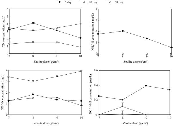
Fig. 4 Effect of bio-zeolite dose on N removal in overlying water.
