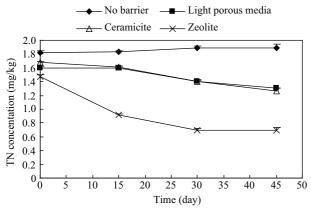
Fig. 2 Effect of cap material type on total nitrogen removal in sediment.
