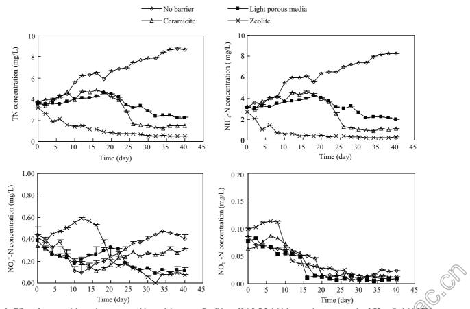
Fig. 1 Effect of cap materials on nitrogen removal in overlying water. Condition: pH 6.5–7.5; initial ammonium concentration 3.75 mg/L; initial TN concentration 3.75 mg/L; temperature 20–25°C.
