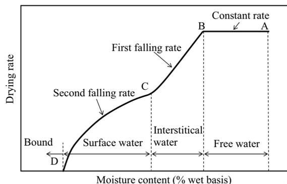
**Fig. 2** Typical sludge drying curve.
