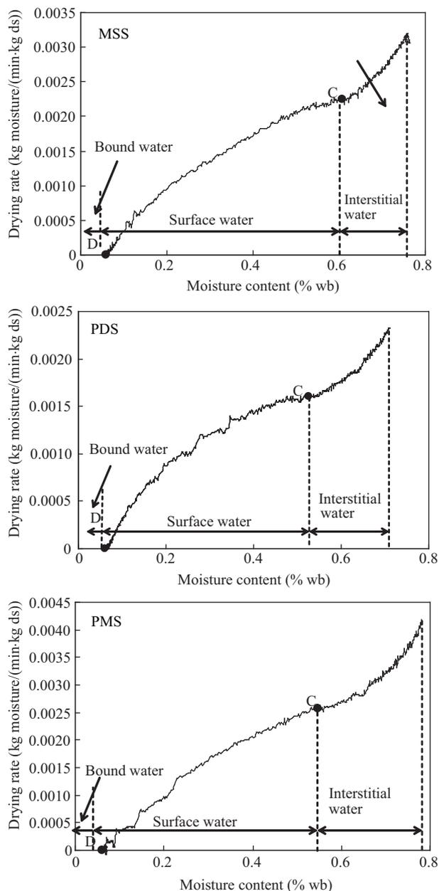
Fig. 3 Drying rate curves of MSS, PDS, and PMS. ds: dry solid; wb: web basis.
