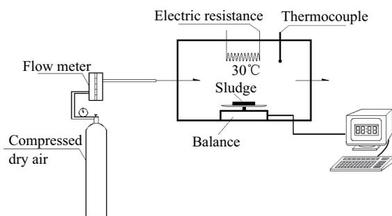
**Fig. 1** Schematic diagram of drying test.
