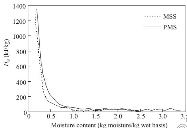
**Fig. 5** Bond strength of moisture in MSS and PMS through TG-DSC test at 90°C.
