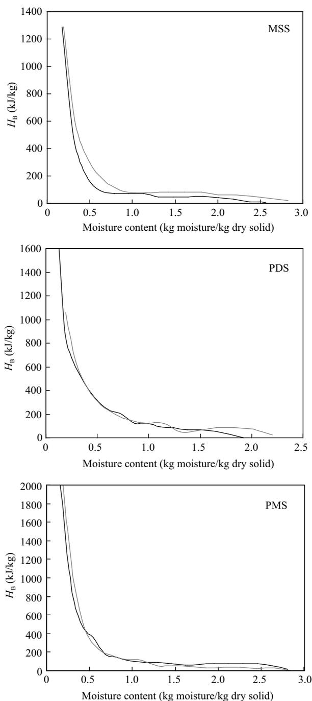
**Fig. 4** Bond strength of moisture in MSS, PDS, and PMS through TG-DTA test at 80°C (two replicates).  $H_B$  is bond strength.
