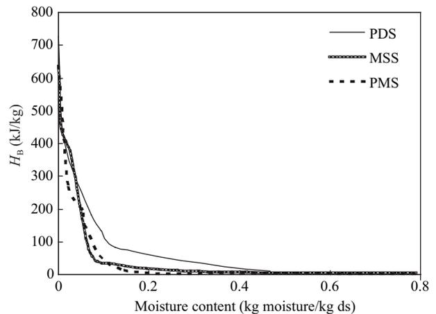
Fig. 6 Bond strength of moisture in MSS, PDS and PMS through water activity test.
