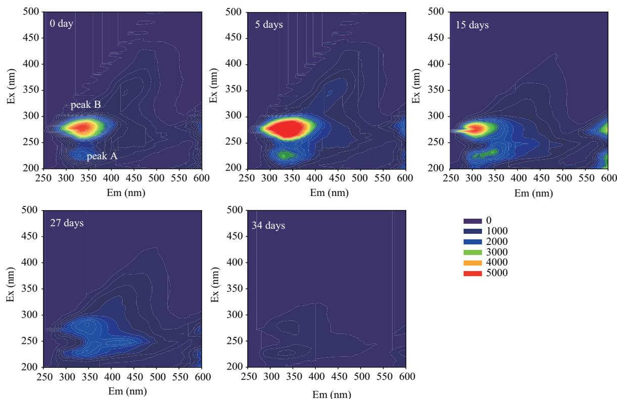
**Fig. 4** Fluorescence EEM of the slime fraction for sonicated sludge.
