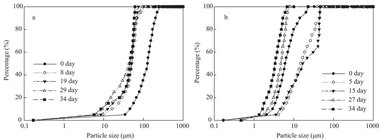
**Fig. 3** Variations of PSD during anaerobic digestion. (a) unsonicated sludge; (b) sonicated sludge.
