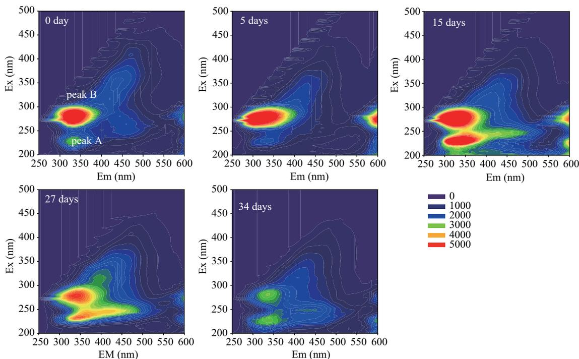
Fig. 5 Fluorescence EEM of the LB-EPS fraction for sonicated sludge.
