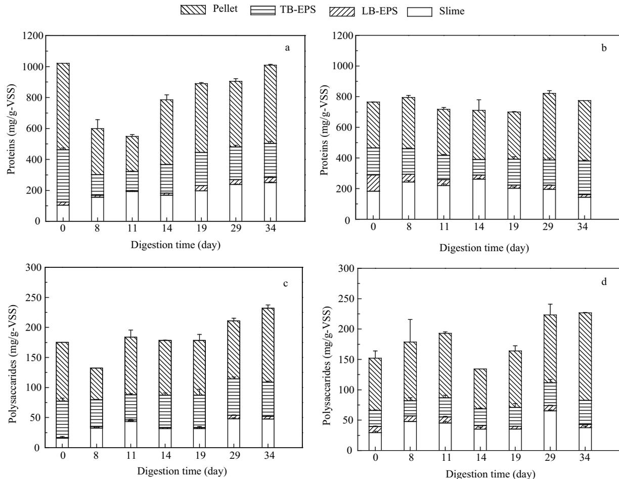
**Fig. 2** Evolutions of organic matters during anaerobic digestion. (a) proteins for unsonicated sludge; (b) proteins for sonicated sludge; (c) polysaccharides for unsonicated sludge; (d) polysaccharides for sonicated sludge.
