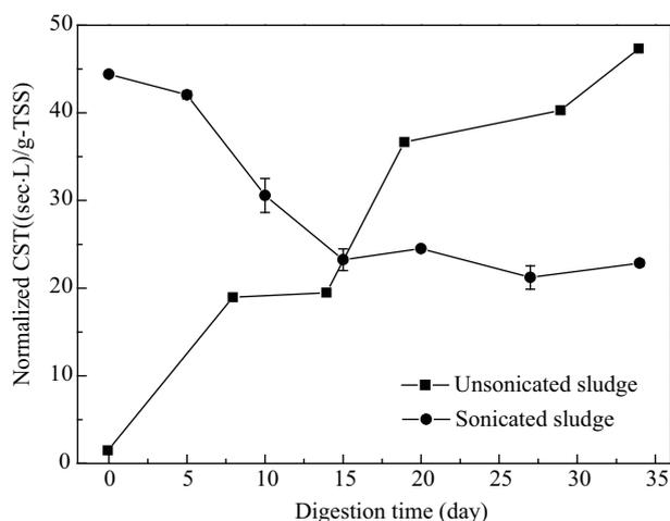
Fig. 1 Variations of sludge dewaterability during anaerobic digestion.
