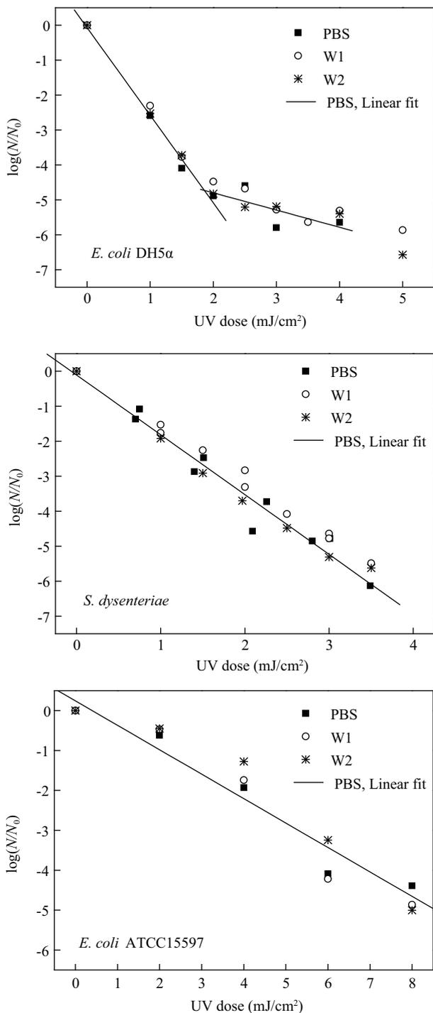
**Fig. 1** UV dose-response curves of the tested bacteria in the three water matrices. W1: the wastewater treated with membrane bioreactor; W2: the wastewater treated with microfilter; PBS: phosphate buffered saline.
