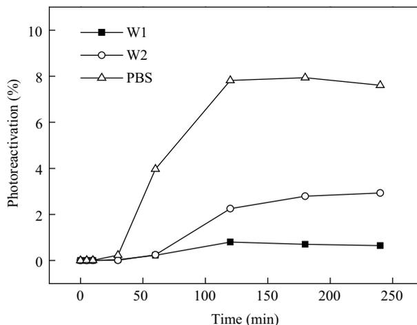
**Fig. 3** Photoreactivation of *E. coli* ATCC15597 after pretreatment with 8 mJ/cm $^2$  UV in different water samples (the fluorescent light intensity at 360 nm was 0.066 mW/cm $^2$ ).
