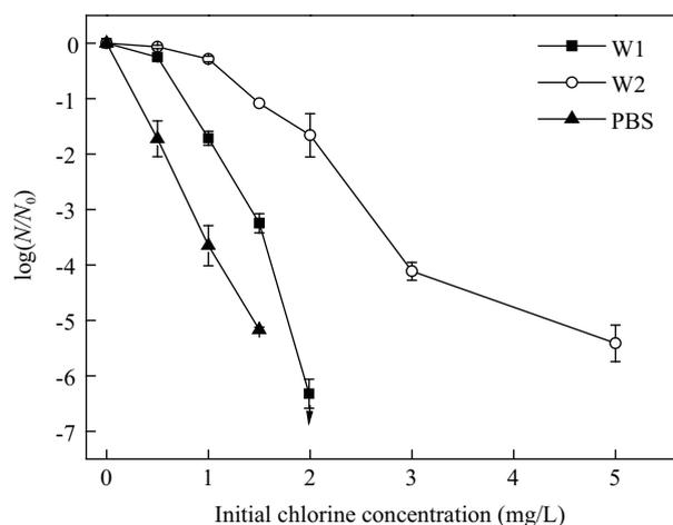
Fig. 5 Effect of water quality on the inactivation of *E. coli* ATCC15597 by chlorine after contact time of 30 min.
