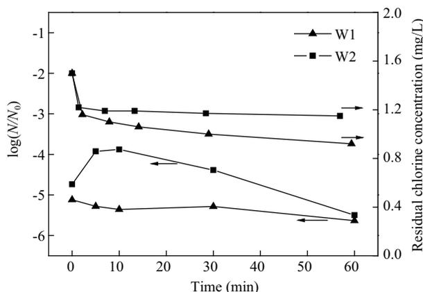
Fig. 7 Inactivation of *E. coli* and chlorine consuming in two filtered wastewater samples with 1.5 mg/L of chlorine after pretreatment with UV of 8 mJ/cm<sup>2</sup>.
