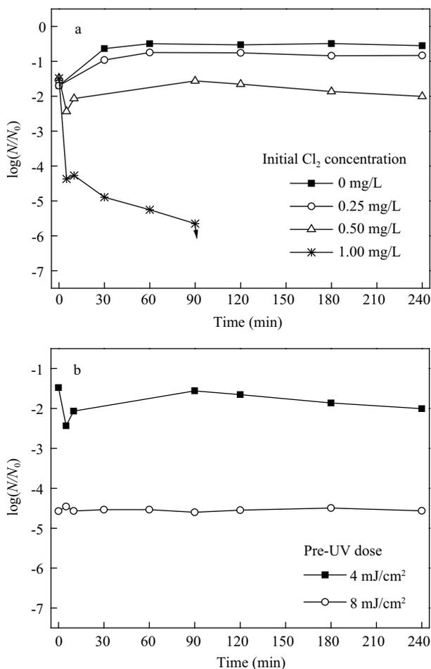
Fig. 6 Inactivation curve of *E. coli* ATCC15597 with different levels of chlorine under fluorescent light after pretreatment with UV of 4 mJ/cm<sup>2</sup> (a) and curve with 0.5 mg/L chlorine under fluorescent light after different levels of UV pretreatment (b) in PBS.
