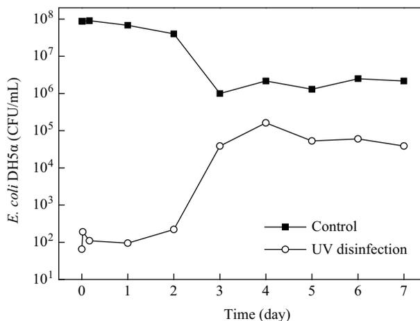
**Fig. 2** *E. coli* DH5 $\alpha$  concentration versus incubation time in dark after pretreatment by UV dose of 8 mJ/cm $^2$  and non-irradiation in W1 sample.
