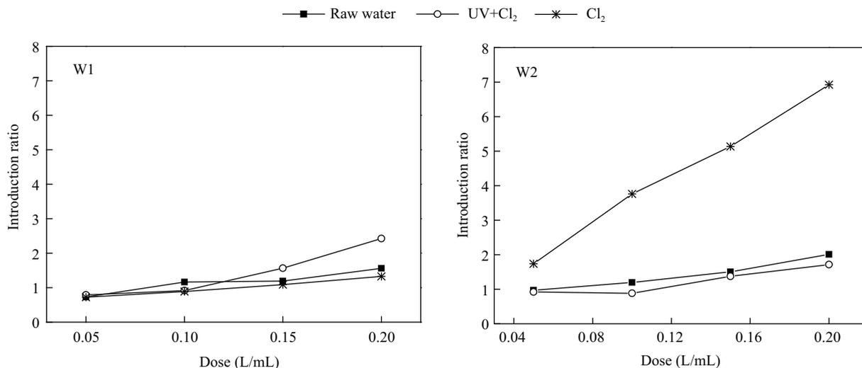
Fig. 8 Genotoxicity changes during different disinfection procedure. UV+Cl<sub>2</sub>: 8 mJ/cm<sup>2</sup> UV irradiation followed by 1.5 mg/L chlorine; Cl<sub>2</sub>: 5 mg/L
