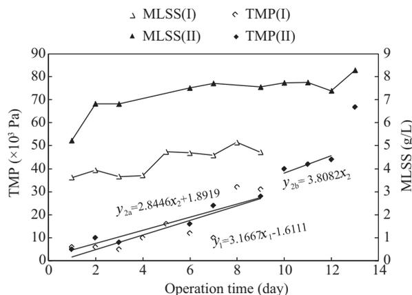
Fig. 2 Changes of trans-membrane pressure (TMP) and mixed liquor suspended solid (MLSS) against operation time. I, II mean first and second operation cycle, respectively.
