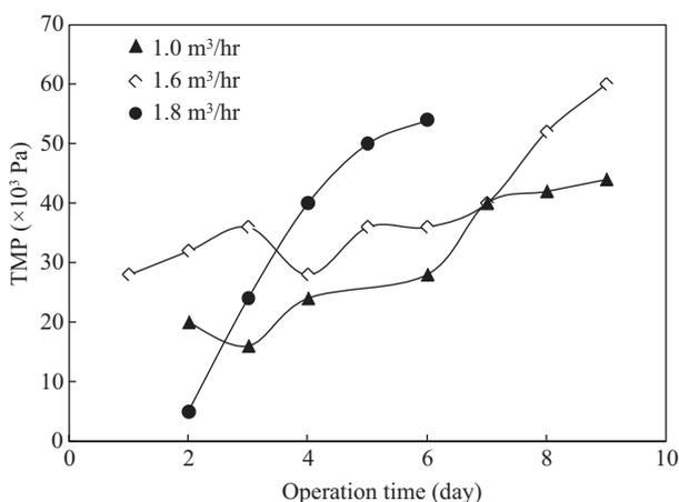
**Fig. 6** Changes of TMP against operation time under different aeration intensity.
