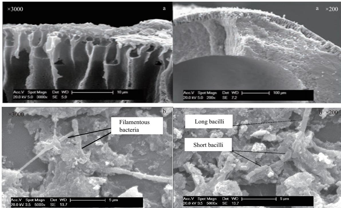
**Fig. 5** Scanning electron microscopy (SEM) micrographs of a polluted membrane thread and the mixture sludge of O zone in A/O MBR system. (a) membrane wire cross-section scan before cleaning; (b) activated sludge micro.
