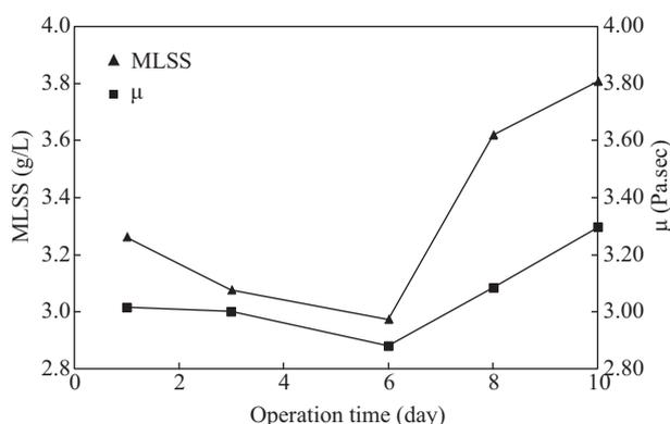
Fig. 3 Changes of MLSS and sludge viscosity ( $\mu$ ) against operation time.
