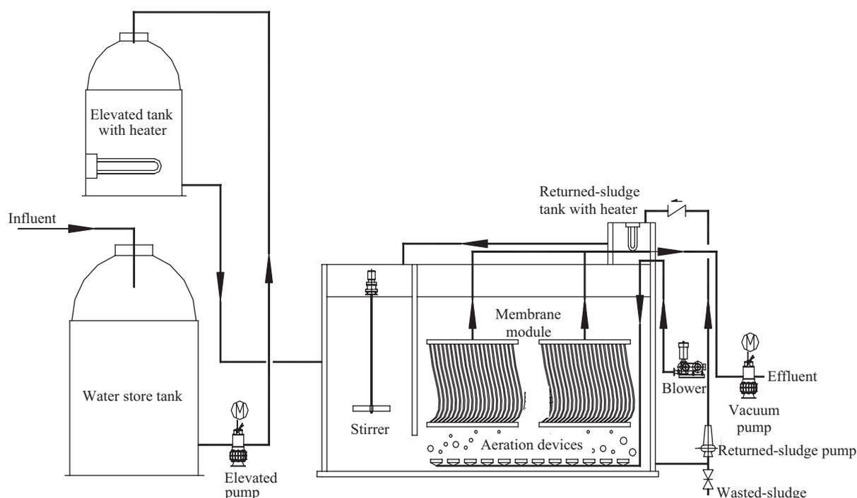
**Fig. 1** Experimental equipments and technical process.
