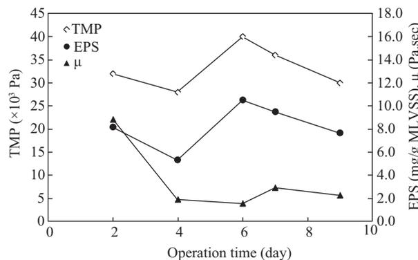
Fig. 4 Changes of extracellular polymeric substance (EPS), TMP and sludge viscosity against operation time.
