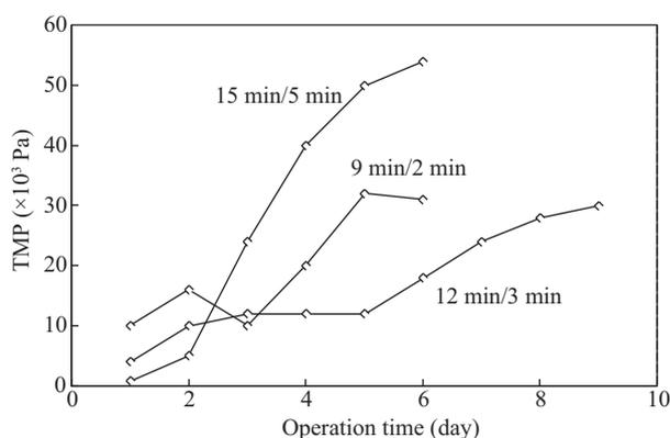
Fig. 8 Changes of TMP against operation time under different suction/suspended time.
