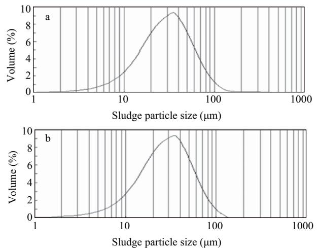
**Fig. 7** Particle size distribution of sludge mixture. Under aeration intensity 1.0 m<sup>3</sup>/hr (a) or 1.6 m<sup>3</sup>/hr (b).
