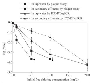
**Fig. 1** Inactivation curves of rotaviruses by chlorine disinfection evaluated by plaque assay and ICC-RT-qPCR assay, either in tap water and secondary effluent matrix, with 60 min exposure time. The arrows indicate detection limits of plaque assay, which had maximum reduction of 3.6 log<sub>10</sub> with initial concentration of  $4 \times 10^3$  PFU/mL rotavirus.
