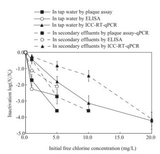
Fig. 3 Reductions of rotaviruses antigencity (ELISA) and infectivity by chlorine disinfection with 60 min exposure in either tap water or secondary effluents.
