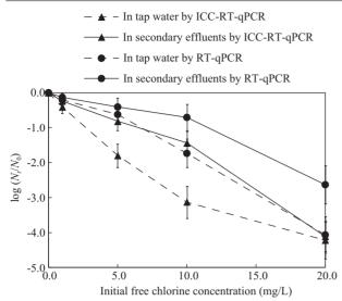
**Fig. 2** Reductions of rotavirus gene (VP7 gene segment, indicative of infectivity) by chlorine disinfection with 60 min exposure, determined by both direct RT-qPCR and ICC-RT-qPCR methods, in either tap water or secondary effluents.
