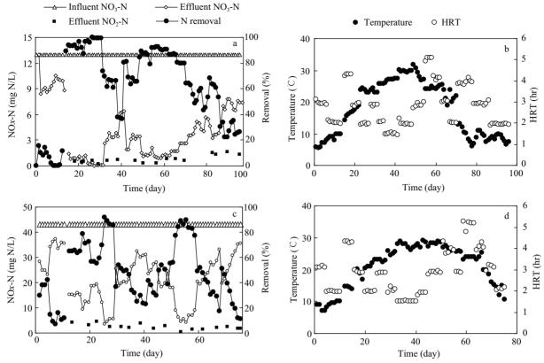
Fig. 2 Running performance of the continuous reactor treating nitrate-contaminated water of 10 mg N/L (a, b) and 40 mg N/L (c, d).
