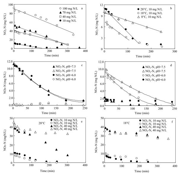
**Fig. 5** Variation of NO<sub>3</sub>-N and/or NO<sub>2</sub>-N in batch test. (a) reduction of NO<sub>3</sub>-N at different initial concentrations; (b) reduction of NO<sub>3</sub>-N at different temperatures; (c) reduction of NO<sub>3</sub>-N under different pH; (d) reduction of NO<sub>2</sub>-N under different pH; (e, f) comparison of NO<sub>3</sub>-N and NO<sub>2</sub>-N reduction rate at 28 and 18°C, respectively.
