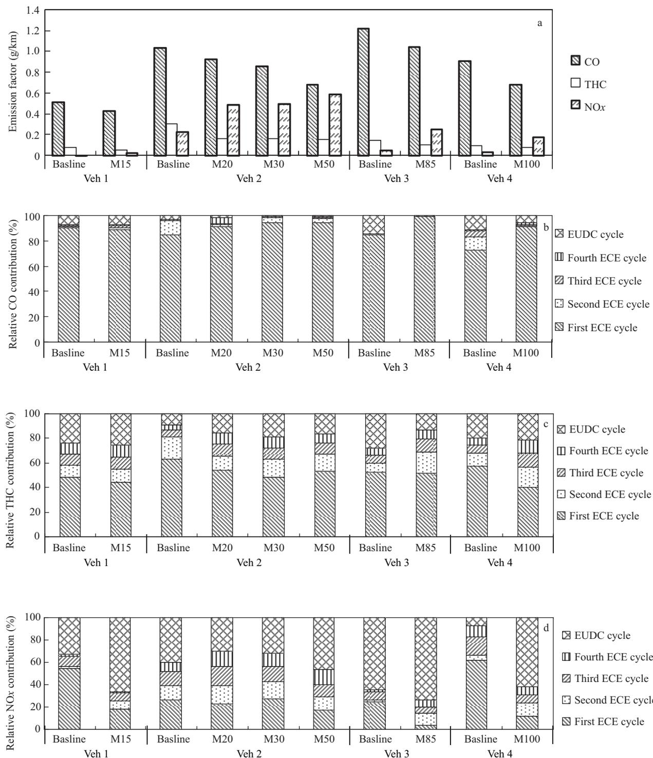
**Fig. 2** Regulated emissions and relative contributions from each stage of the test cycle. (a) regulated emissions; (b) relative CO contribution; (c) relative THC contribution; (d) relative NO<sub>x</sub> contribution.
