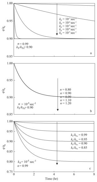
**Fig. 3** Predicted effect of  $k_d$  (a), n (b), and  $k_F/k_{Fe}$  (c) on the desorption of adsorbate from adsorbent.
