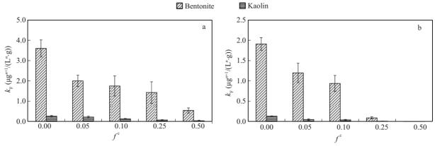
Fig. 2 Adsorption capacity of bentonite and kaolin for: (a) benzene and (b) toluene.
