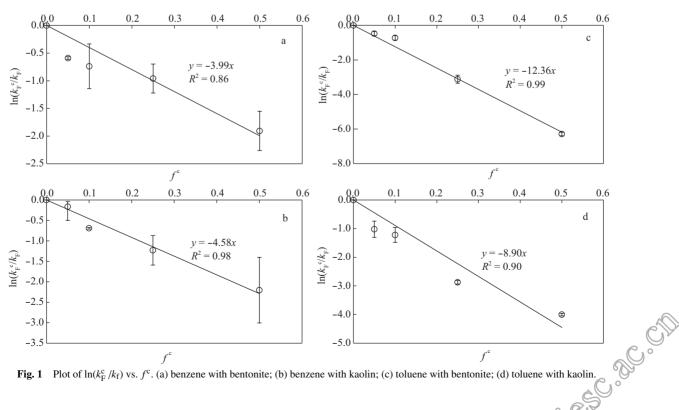
**Fig. 1** Plot of  $\ln(k_F^c/k_f)$  vs.  $f^c$ . (a) benzene with bentonite; (b) benzene with kaolin; (c) toluene with bentonite; (d) toluene with kaolin.
