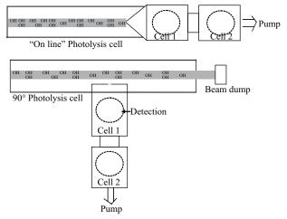
Fig. 2 Kinetic configurations schemes for the laser photolysis cell: upper graph on line configuration (OLC), lower graph  $90^{\circ}$  configuration (NDC).
