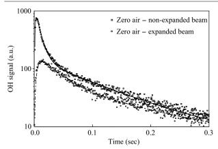
**Fig. 3** Comparison between two OH time decay profiles in zero air in the NDC: Non-expanded beam, expanded beam. The solid line corresponds to a fit using a double exponential decay,  $k'_0$ =9.72 sec<sup>-1</sup>. The dashed line represents a fit using a single exponential decay,  $k'_0$  = 13.86 sec<sup>-1</sup>.
