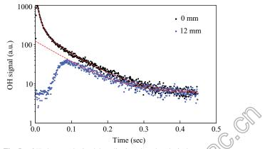
Fig. 5 OH decays obtained by aligning the photolysis laser at two different positions with respect to the inlet nozzle.
