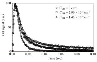
Fig. 4 OH decays for 3 different  $CH_4$  concentrations, obtained in the NDC with non-expanded beam.
