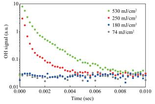
Fig. 6 Interference generation of OH radicals through impact of photolysis laser beam onto the metal nozzle in the OLD configuration.
