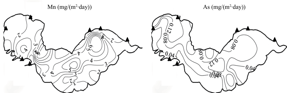
Fig. 8 Contour map of Mn and As diffuse flux from pore water to overlying water.
