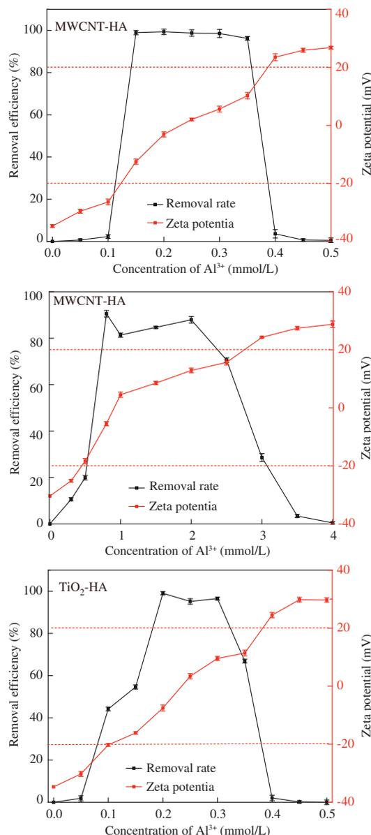
**Fig. 1 – Removal rate and zeta potential of nanoparticles varied with the dosage of Al<sup>3+</sup>.**
