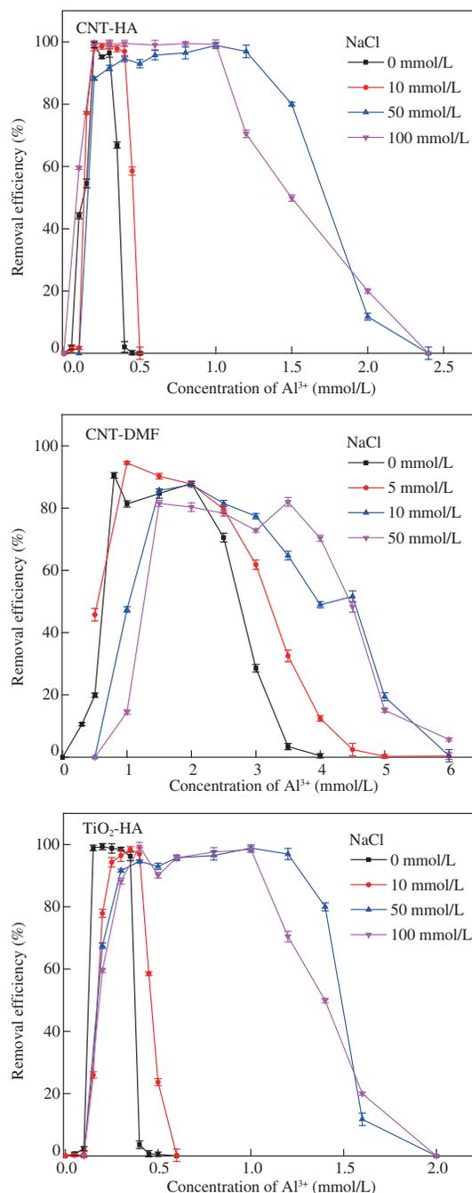
**Fig. 3 – Effect of ionic strength on nanoparticle coagulation removal, pH = 7 ± 0.1. The ECR becomes broader with increasing ionic strength of NaCl.**
