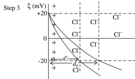
**Fig. 4 – Schematic model of the effect of ionic strength on nanoparticle coagulation.**
