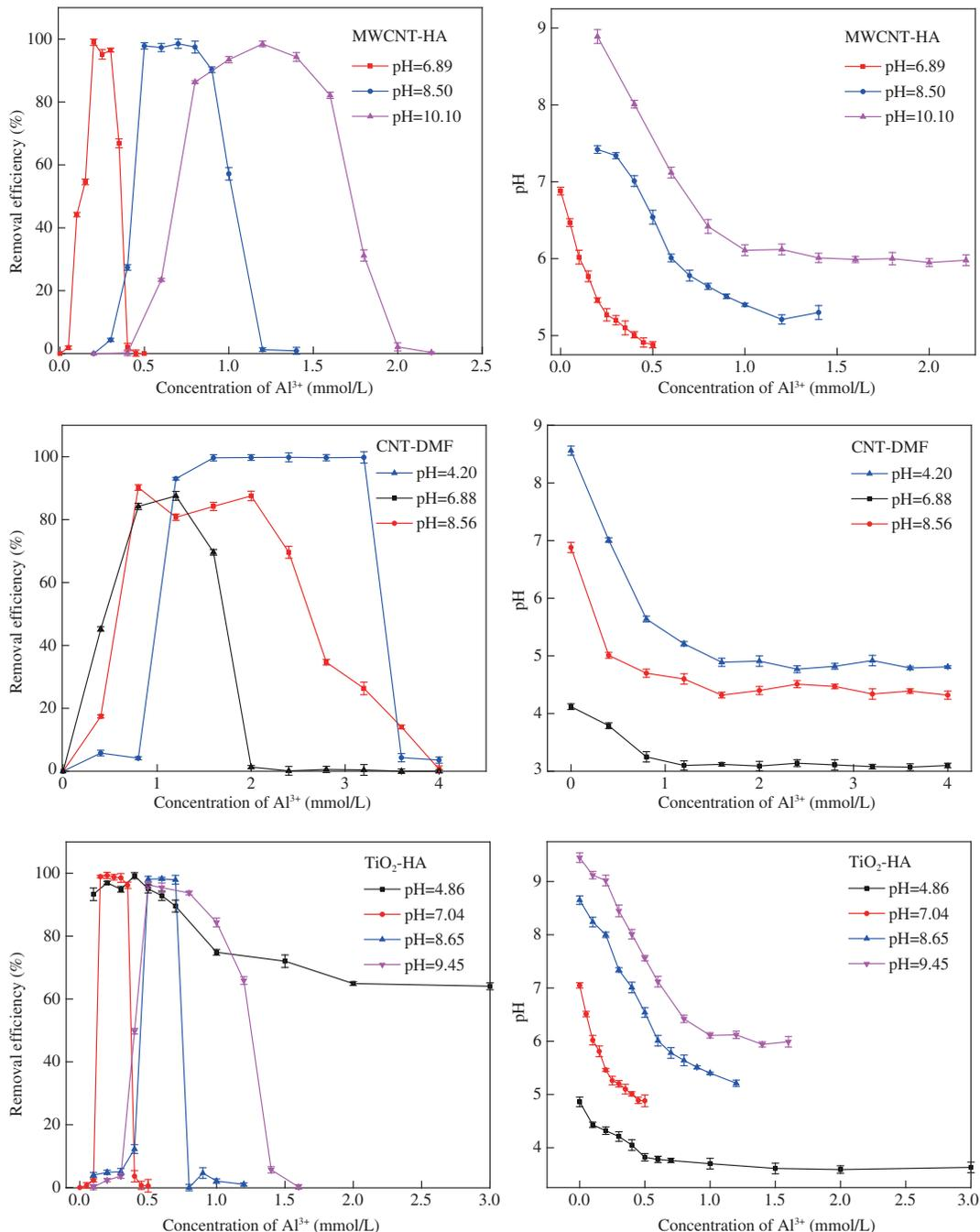
Fig. 2 – Changes of effective concentration range (ECR) of Al<sup>3+</sup> at different pH. The left figures showed ECR in acid condition, neutral condition and basic condition, pH was measured after coagulation.
