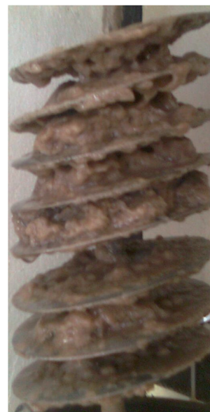
Fig. 1 – Filling of sequencing batch biofilm reactor (SBBR) with biofilm.
