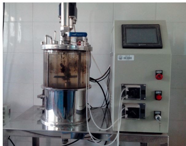
Fig. 1 – Semi-continuously operated two-phase anaerobic digested reactor (single SCFA-production or gas-production reactor). SCFA: short-chain fatty acid.
