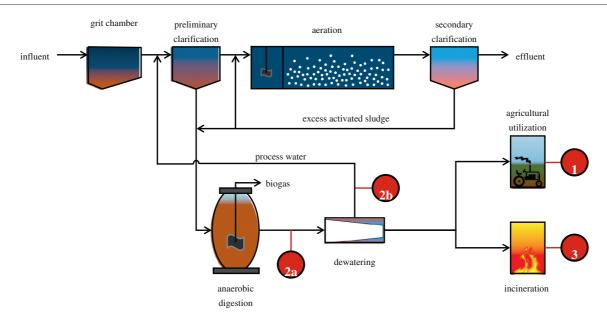
Fig. 3 – Hot spots for P recovery in wastewater treatment plant (Kabbe and Remy, 2013). 1. Direct agricultural utilization of dewatered sludge; 2a. undrained sludge after anaerobic digestion; 2b. sludge liquor after dewatering; 3. from ash after undiluted incineration.
