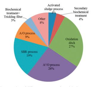
Fig. 2 – Variety of different processes of municipal wastewater treatment plants in China.
