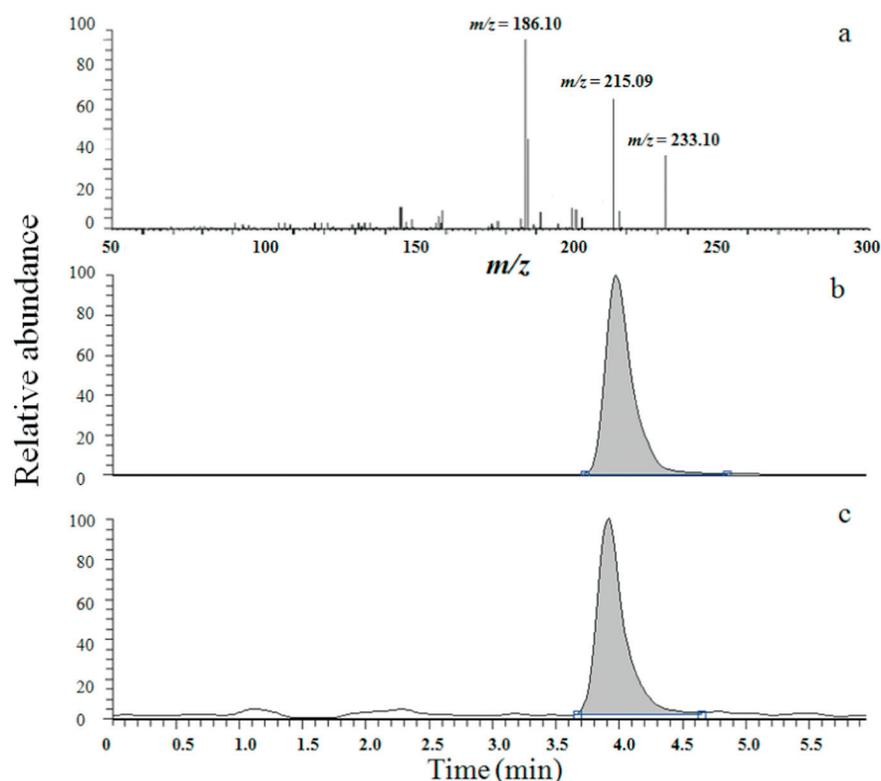
**Fig. 1 – (a) ESI-MS/MS analysis of the derivatization product of 4,5-dihydroxy-2,3-pentanedione (DPD); (b) typical chromatogram of blank Luria-Bertani (LB) medium spiked with DPD at 10 ng/mL; and (c) typical chromatogram of a real biological sample. The product ion  $m/z = 186.10$  was used for quantification.**
