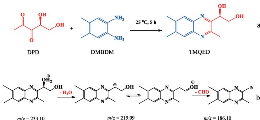
**Scheme 1 – (a) Derivatization of 4,5-dihydroxy-2,3-pentanedione (DPD) with 4,5-dimethylbenzene-1,2-diamine (DMBDM) for electrospray ionization tandem mass spectrometry (ESI-MS/MS) analysis; TMQED: 1-(3,6,7-trimethylquinoxalin-2-yl)ethane-1,2-diol; and (b) ESI-MS/MS fragmentation schemes of the derivatization product (TMQED).**
