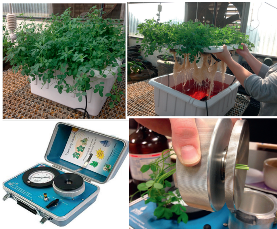
Fig. 1 – Hydroponic system with fully grown alfalfa plants with its root zone and the nutrient solution. Schematic shows the Model 600 Pressure Chamber Instrument with the sap extraction in progress.
