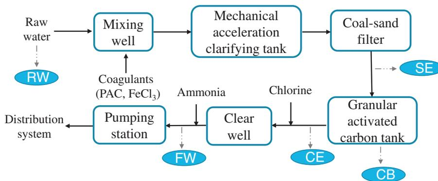
**Fig. 1 – Schematic diagram of the drinking water treatment process. RW: raw water; SE: coal-sand filter effluent; CB: GAC particles; CE: GAC tank effluent; FW: finished water; GAC: granular activated carbon.**
