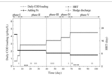
Fig. 2 - Different operating conditions of IUSR.
