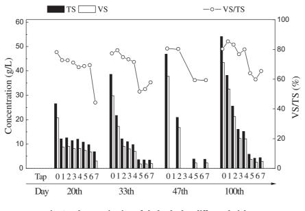
Fig. 6 - Characterization of sludge bed at different heights.
