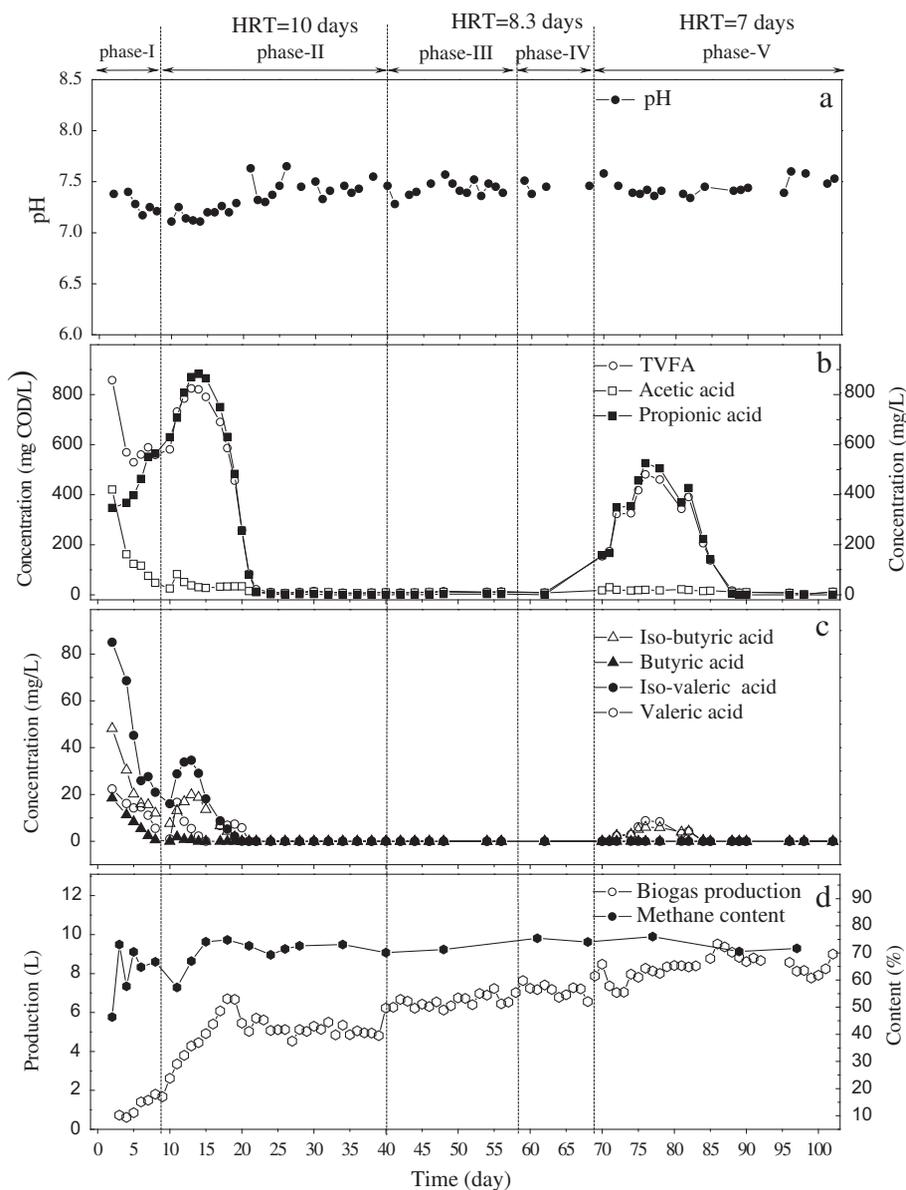
**Fig. 3 – Performance of IUSR under different operating conditions. a: pH; b and c: TVFA and VFAs; d: biogas production and methane content.**
