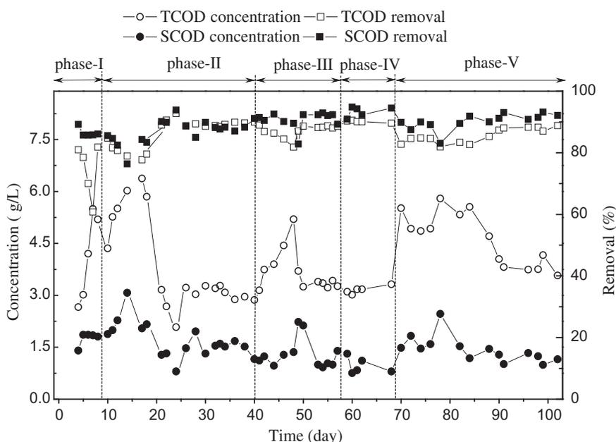
**Fig. 4 – COD concentrations of effluents and COD removal under different operating conditions.**
