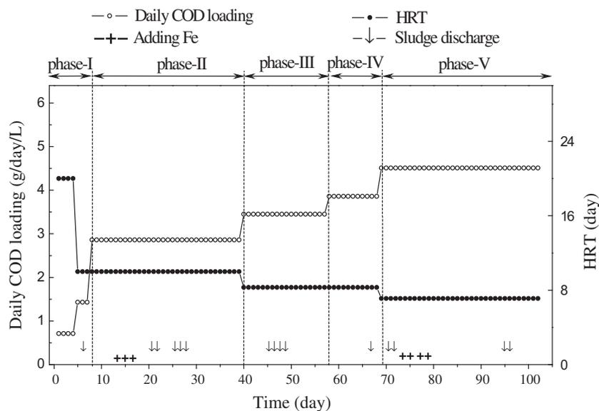
Fig. 2 – Different operating conditions of IUSR.
