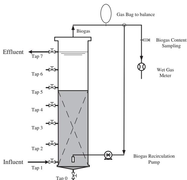
**Fig. 1 – Schematic diagram of an improved upflow solid reactor (IUSR).**
