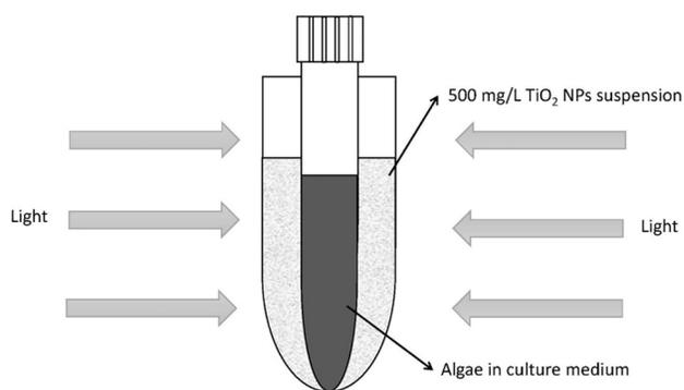
**Fig. 1 – Diagram of shading effect of 500 mg/L TiO<sub>2</sub> nanoparticles on microalgae.**
