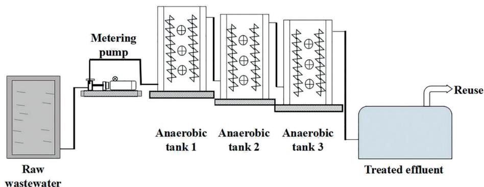
Fig. 1 – Schematic drawing of anaerobic biofilm reactor.
