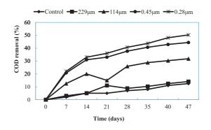
Fig. 4 – Chemical oxygen demand removal efficiencies under varying interface layer pore sizes.
