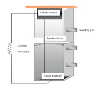
Fig. 1 – Schematic representation of the single-chamber sediment microbial fuel cells employed in the study.
