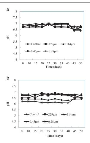
Fig. 2 – Cathodic pH variations with respect to interface layer pore sizes (a) and anodic pH variations according to the porosity of the interface layer (b).
