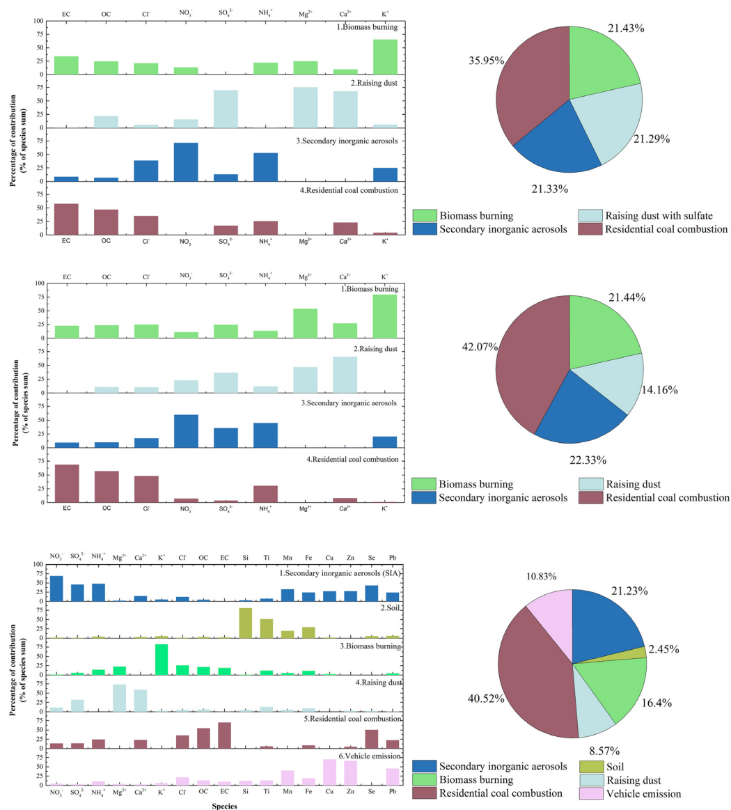
Fig. 5 – Results of PMF (positive matrix factor) analysis with 9 species during (a) pre-heating and (b) heating period in DBT rural area and (c) results of PMF analysis with 17 species during heating period in DBT rural area.
