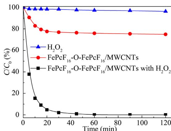
**Fig. 3 – Degradation of carbamazepine (CBZ) under different conditions. Reaction conditions:  $C_0 = 2.5 \times 10^{-5}$  mol/L, concentration of  $H_2O_2$  ( $[H_2O_2]$ ) =  $5 \times 10^{-3}$  mol/L, concentration of FePcF<sub>16</sub>-O-FePcF<sub>16</sub>/MWCNTs ( $[FePcF_{16}-O-FePcF_{16}/MWCNTs]$ ) = 0.2 g/L, temperature ( $T$ ) = 303.15 K and pH 7.  $C_0$ : initial concentration of CBZ;  $C$ : concentration of CBZ at time  $t$ .**
