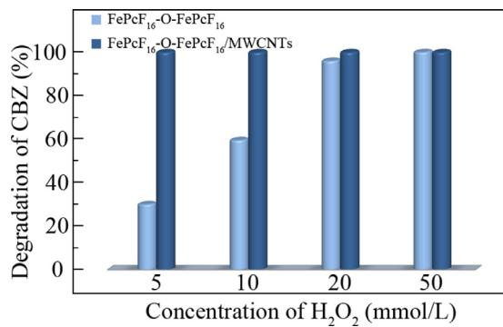
**Fig. 5 – Effect of initial  $\text{H}_2\text{O}_2$  concentration on catalytic degradation of CBZ different conditions. Reaction conditions:  $C_0 = 2.5 \times 10^{-5} \text{ mol/L}$ ,  $T = 323.15 \text{ K}$ , pH 7,  $[\text{FePcF}_{16}\text{-O-FePcF}_{16}] = 0.1 \text{ g/L}$  or  $[\text{FePcF}_{16}\text{-O-FePcF}_{16}/\text{MWCNTs}] = 0.2 \text{ g/L}$ .**
