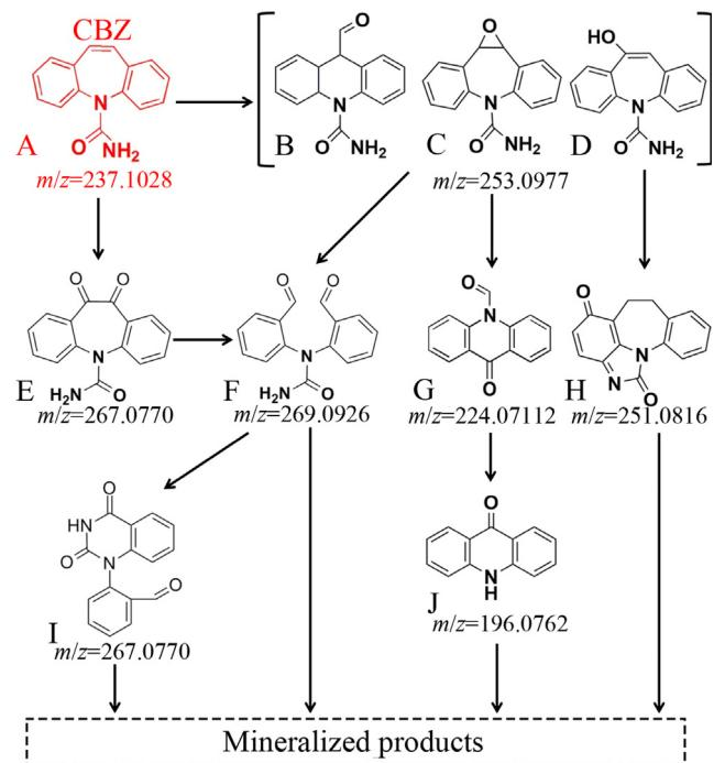
**Fig. 8 – Proposed CBZ degradation pathway in the FePcF<sub>16</sub>-O-FePcF<sub>16</sub>/MWCNTs/H<sub>2</sub>O<sub>2</sub> system.**
