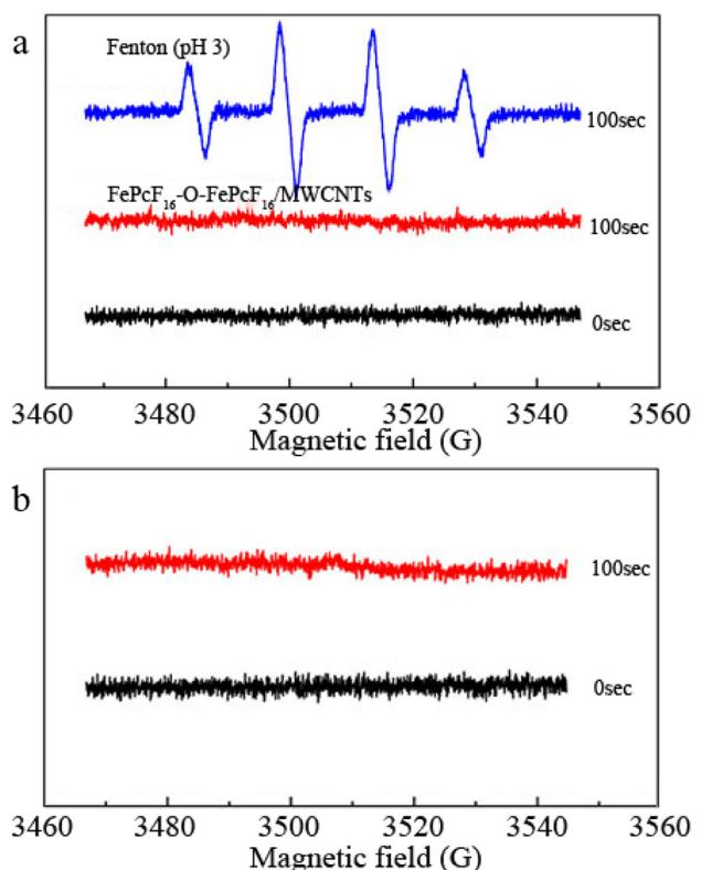
**Fig. 6 – 5,5-Dimethyl-1-pyrroline N-oxide (DMPO) spin-trapping electron paramagnetic resonance (EPR) spectra in (a) pure aqueous solution or (b) methyl alcohol solutions with  $[\text{H}_2\text{O}_2] = 5 \times 10^{-3} \text{ mol/L}$ , concentration of DMPO ( $[\text{DMPO}] = 5 \times 10^{-3} \text{ mol/L}$ ,  $[\text{FePcF}_{16}\text{-O-FePcF}_{16}/\text{MWCNTs}] = 0.2 \text{ g/L}$ .**
