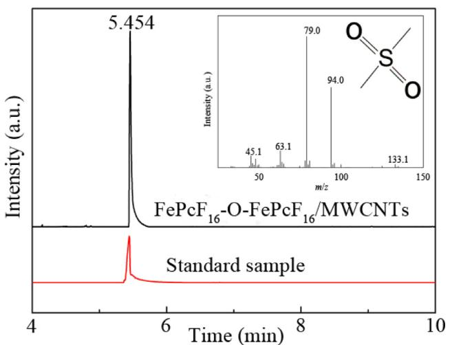
**Fig. 7 – Gas chromatography mass spectrometry (GC-MS) chromatograms of dimethyl sulfone ( $\text{DMSO}_2$ ) ( $1 \times 10^{-3} \text{ mol/L}$ ), oxidation products of dimethyl sulfoxide (DMSO) catalyzed by  $\text{FePcF}_{16}\text{-O-FePcF}_{16}/\text{MWCNTs}$ . Inset shows the MS spectrum of  $\text{DMSO}_2$ .  $m/z$ : mass-to-charge ratio.**
