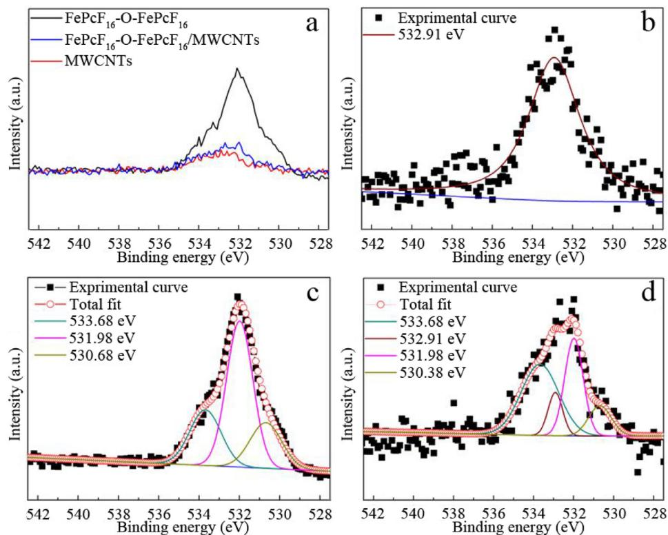
**Fig. 2 – Curves of O1s peaks of (a) MWCNTs, FePcF<sub>16</sub>-O-FePcF<sub>16</sub> and FePcF<sub>16</sub>-O-FePcF<sub>16</sub>/MWCNTs, (b) MWCNTs, (c) FePcF<sub>16</sub>-O-FePcF<sub>16</sub> and (d) FePcF<sub>16</sub>-O-FePcF<sub>16</sub>/MWCNTs.**
