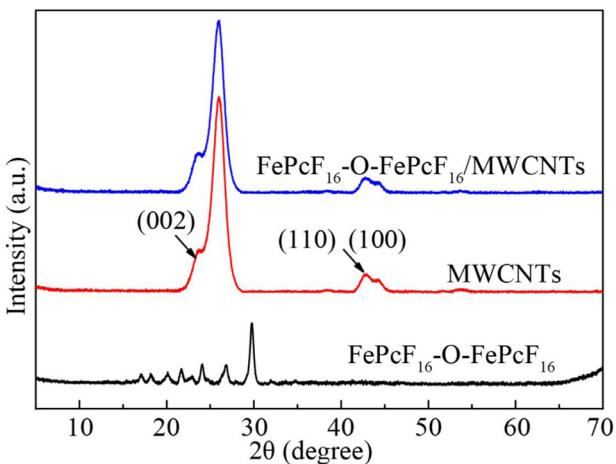
**Fig. 1** – Powder X-ray diffraction diagrams of O-bridged iron perfluorophthalocyanine dimers ( $\text{FePcF}_{16}\text{-O-FePcF}_{16}$ ), multi-walled carbon nanotubes (MWCNTs) and  $\text{FePcF}_{16}\text{-O-FePcF}_{16}/\text{MWCNTs}$ .
