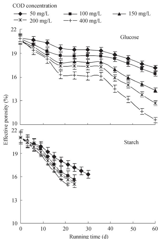
**Fig. 3** Effective porosity as a function of time in glucose-fed and starch-fed systems.
