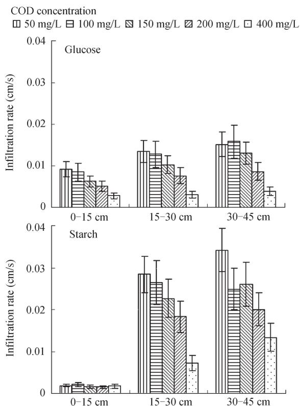
**Fig. 6** Infiltration rates in each layer of systems fed with different organic influents.
