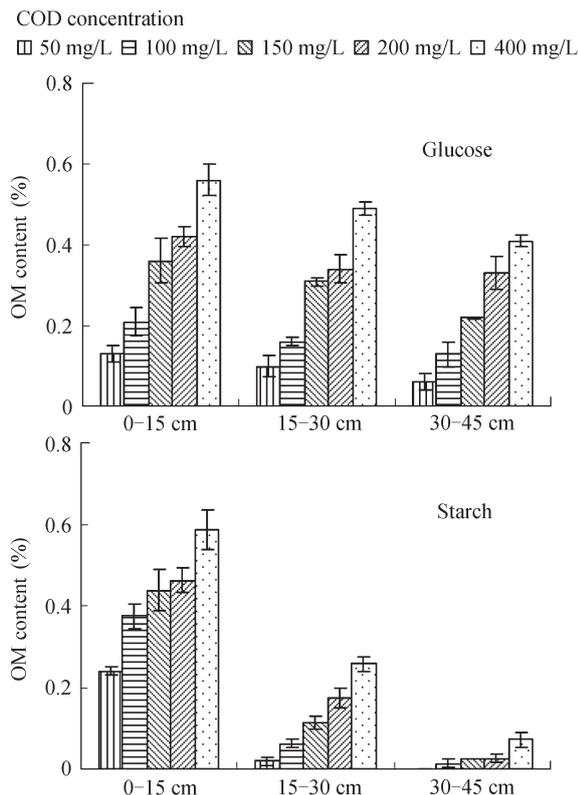
**Fig. 5** Accumulated organic matter (OM) contents in each layer of glucose-fed and starch-fed systems.
