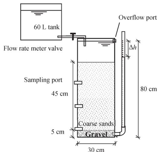
Fig. 1 Schematic description of the experimental vertical flow constructed wetland (VFCW) model.
