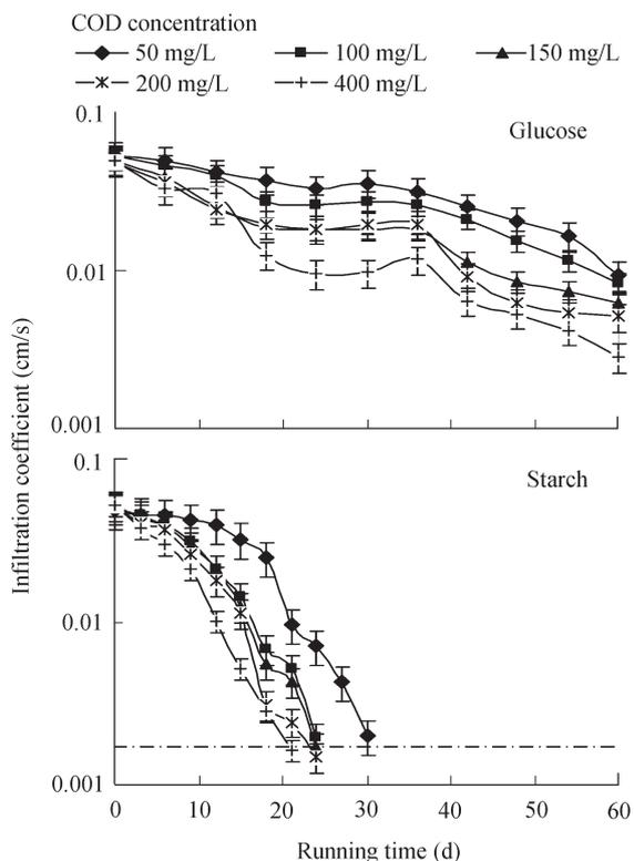
**Fig. 2** Infiltration rate as a function of time in glucose-fed and starch-fed systems.
