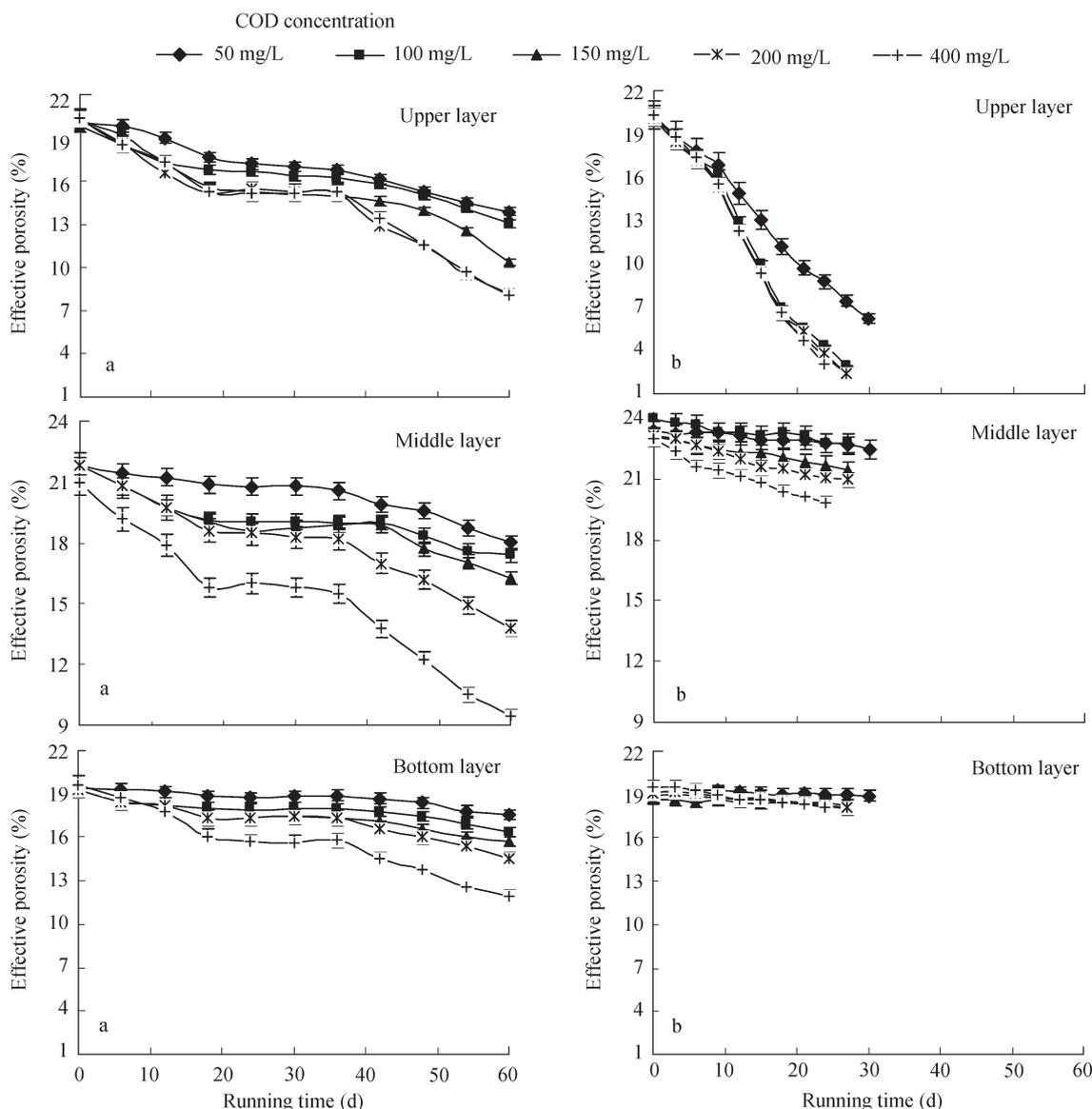
**Fig. 4** Effective porosities of each layer as a function of time in glucose-fed (a) and starch-fed (b) systems.
