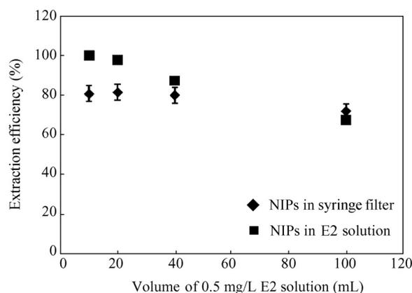
**Fig. 4** Extraction efficiencies for 0.5 mg/L E2 in water using 10 mg of NIP particles prefilled inside a syringe filter or added directly into water.
