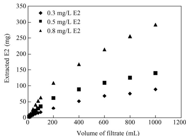
**Fig. 3** Masses of E2 extracted from different volumes of water containing 0.8, 0.5 and 0.3 mg/L E2, using 10 mg of NIP particles inside a syringe filter.
