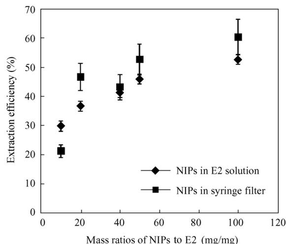
**Fig. 1** Extraction of 1 mg/L E2 (25 mL of water containing 25 g of E2) by NIP particles added directly into water and pre-filled inside a syringe filter. VIP: non-imprinted polymer.
