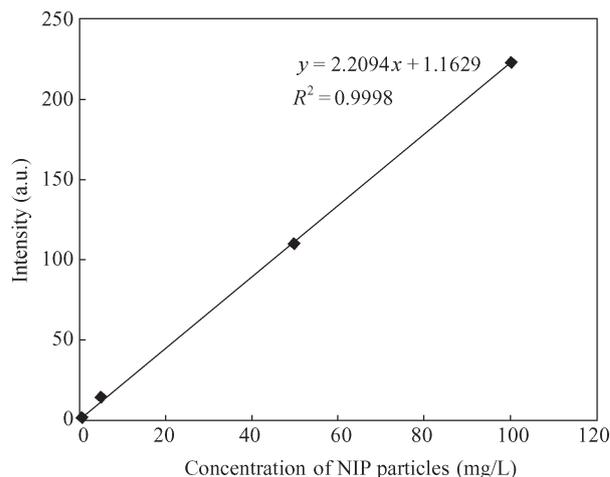
**Fig. 5** Standard calibration curve of light scattering intensity versus concentration of NIP particles in water.
