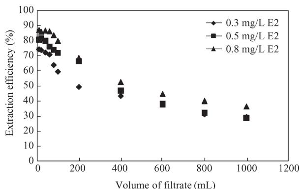
**Fig. 2** Extraction efficiencies for 0.8, 0.5 and 0.3 mg/L E2 in water using 10 mg of NIP particles inside a syringe filter.
