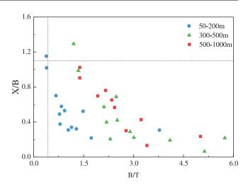
Fig. 5 – Aging extent assessment of air mass using X/B (xylene/benzene) and B/T (benzene/toluene) ratios at different heights 50-200, 300-500 and 500-1000 m.
