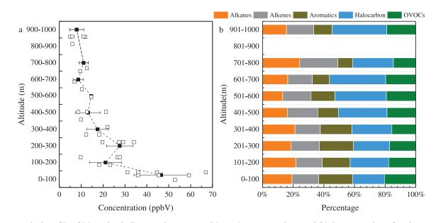
Fig. 3 – Vertical profile of (a) total volatile organic compound (TVOC) concentrations and (b) the proportion of each VOC category at different height ranges. OVOCs: oxygenated volatile organic compounds.
