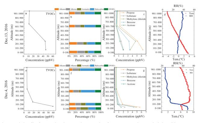
Fig. 4 – Vertical profile of TVOC, selected VOC species, proportion of VOC category, and meteorological conditions (temperature and relative humidity) at noon for two selected flights. (a), (b), (c) and (d) are the result on December 13, 2016 (11:50-12:23,  $PM_{2.5} = 90 \mu g/m^3$ ); (e), (f), (g) and (h) are the result on December 4, 2016 (13:25-13:58,  $PM_{2.5} = 261 \mu g/m^3$ ).
