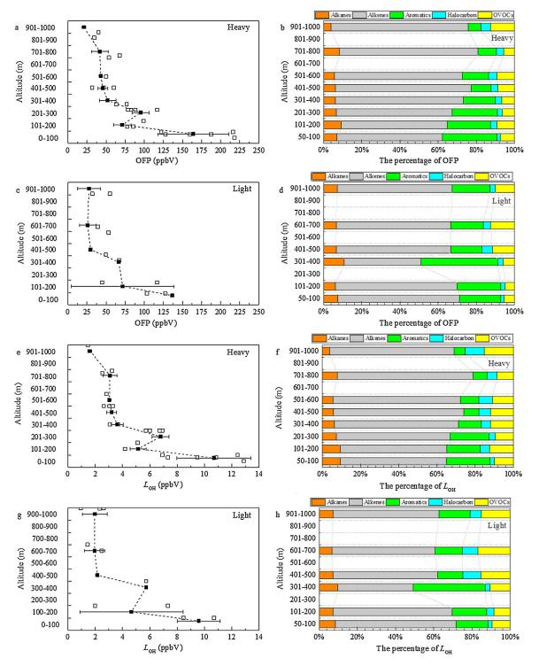
Fig. 6 – Vertical profiles of ozone formation potential (OFP) and OH loss rate ( $L_{OH}$ ) during heavy and light pollution days. (a), (c), (e) and (g) are the vertical profiles of OFP or  $L_{OH}$  of TVOCs, and (b), (d), (f) and (h) are the vertical profile of the proportion of each VOC category in the OFP or  $L_{OH}$  of TVOCs.
