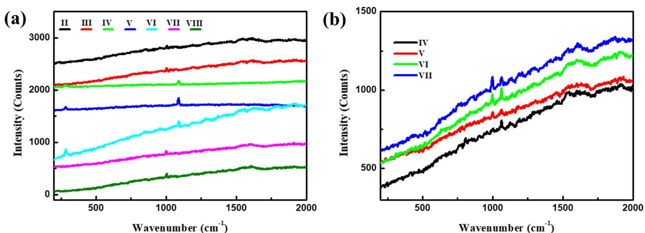
**Fig. 4 – SERS spectra of atmospheric aerosol particles collected by grading particle sampler (a); the optimized SERS spectra from grading IV to VII (b).**
