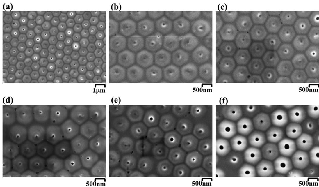
**Fig. 1 – (a)** Top-view SEM images of the Au nanorings; SEM images of different sputtering duration: **(b)** 30 sec, **(c)** 180 sec, **(d)** 240 sec, **(e)** 300 sec, **(f)** 420 sec.
