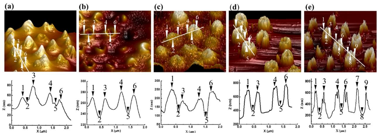
**Fig. 2 – AFM topographic and representative line scan images of the Au nanoring submonolayer at different sputtering duration of the fabrication process. (a)** 30 sec, **(b)** 180 sec, **(c)** 240 sec, **(d)** 300 sec, and **(e)** 420 sec. All arrows marked in the topographic images correspond to the arrows in the line scan images.
