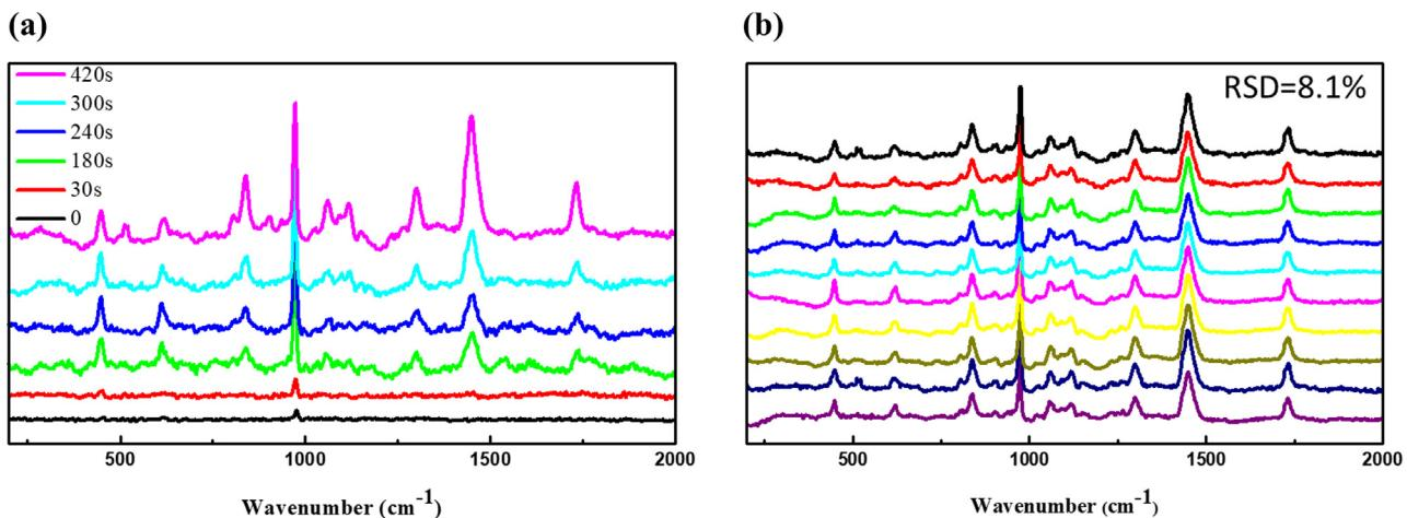
**Fig. 3 – SERS spectra of Au Nanorings with different sputtering duration (a); ten times of SERS measurements using identical Au Nanorings as the substrate and the same (NH<sub>4</sub>)<sub>2</sub>SO<sub>4</sub> aerosols as analyte (b).**
